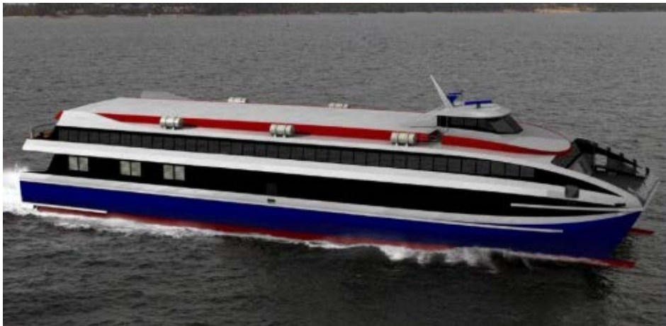
figure H.7 – the Damen Fast Ropax 6016. dimensions: 60x16.2x2.0 m 3 maximum speed: 35.0 kn capacity: 660 passengers and 49 cars
