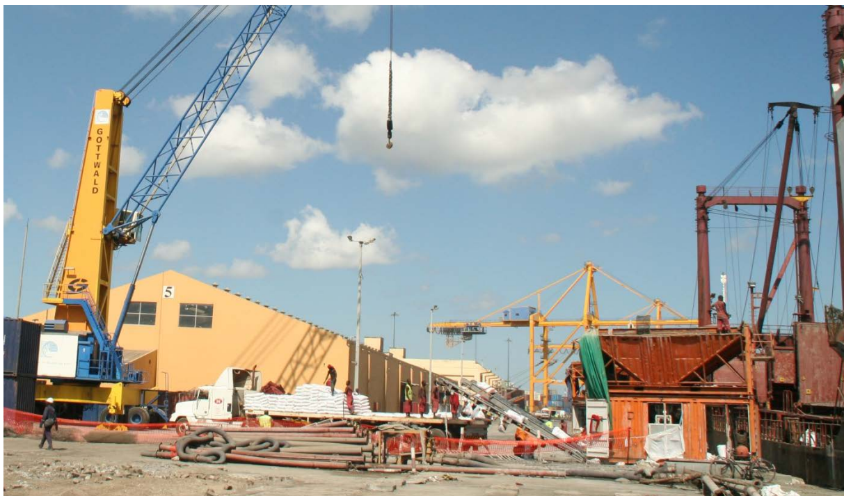
Figure 3-10 | View from quay 8 on unloading activities at quay 7, with 50 T crane and bagging machine
