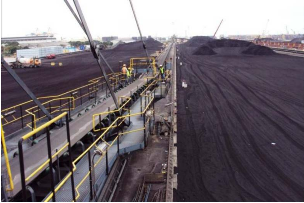
Figure 3-14 | Coal conveyor belt of Beira Port with coal storage on both sides
