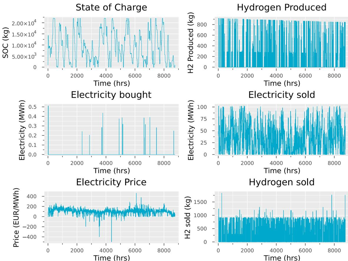
**Figure 5.6:** Time-series plots showing the operational dynamics of the hydrogen production system over a one-year rolling horizon simulation with double the degradation values
