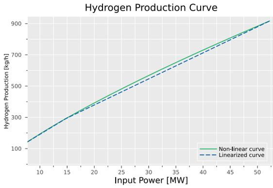
**Figure 4.9:** Non-linear hydrogen production curve without degradation
