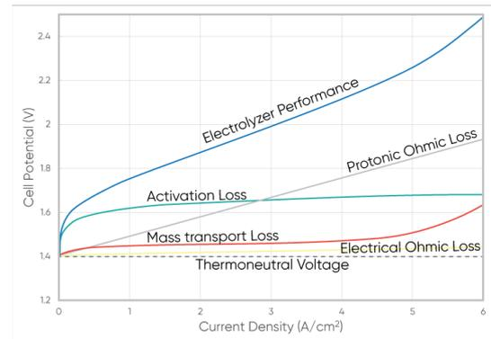
**Figure 3.3:** Detailed polarization curve highlighting activation, ohmic, and concentration overpotentials [55].
