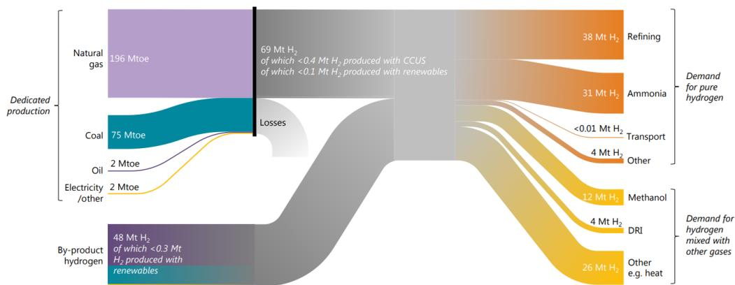
**Figure 1.1:** Flow of hydrogen from energy source to various end-uses[1]
