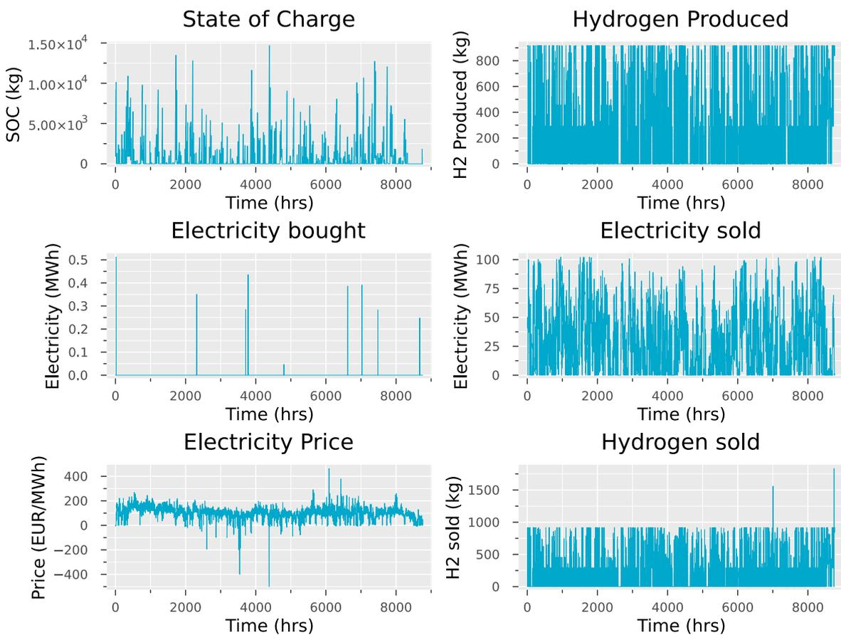
**Figure 5.7:** Simulation results of the rolling horizon approach with a premium implemented and nodegradation implemented. EHB hydrogen premium of €2/kg H<sub>2</sub>
