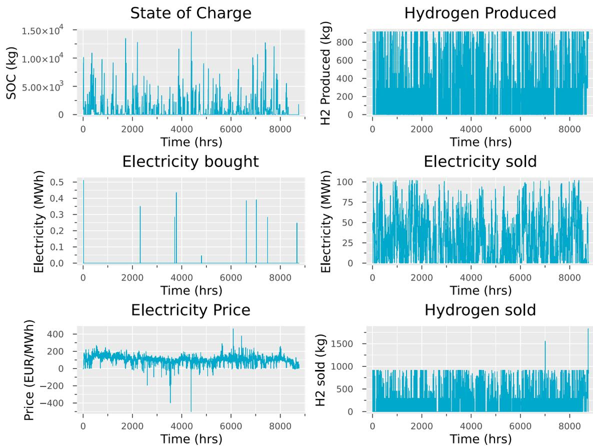
**Figure 5.8:** Rolling horizon approach and hydrogen premium of €4/kg of hydrogen
