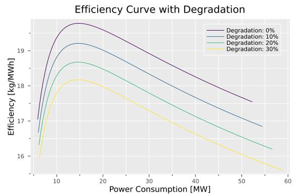
**Figure 4.13:** Effect of degradation on the efficiency curve
