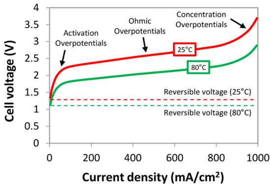
**Figure 3.2:** Polarization curve of an alkaline electrolyzer under varying temperatures, showing reduced losses at higher temperatures [54].
