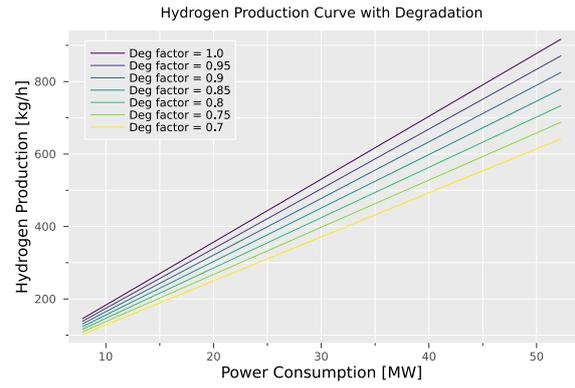
**Figure 4.10:** Shifted hydrogen production curve with degradation
