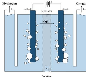
**Figure 3.1:** Simplified schematic of an Alkaline Electrolyzer (AEL) illustrating the basic setup and ion flow [51]
