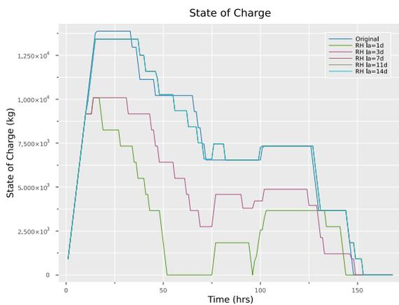
**Figure 5.2:** State of Charge (SOC) comparison between original and rolling horizon scenarios.
