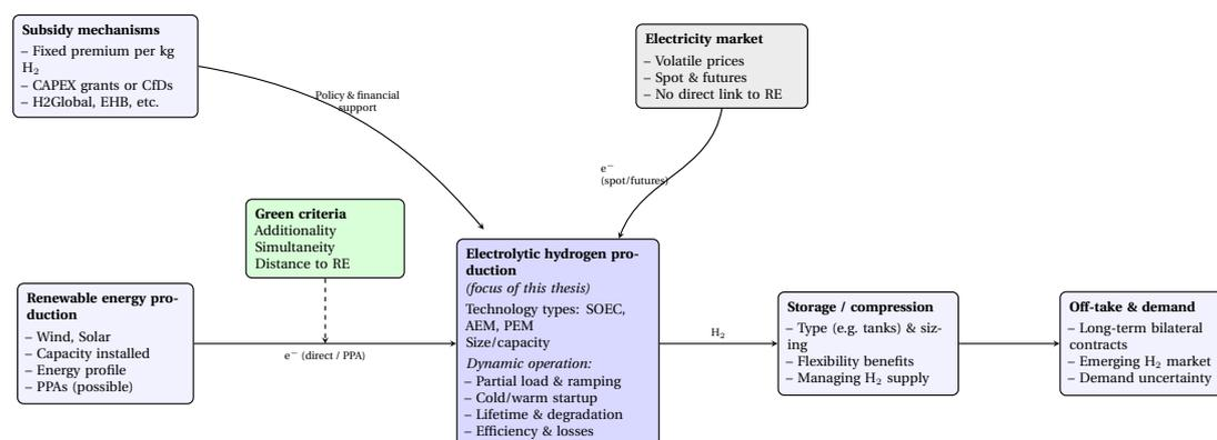
**Figure 1.2:** A simplified schematic of hydrogen production within a renewable energy system, illustrating the central role of the electrolyser in relation to multiple electricity sources, policy support initiatives, storage options, and enduse offtake.
