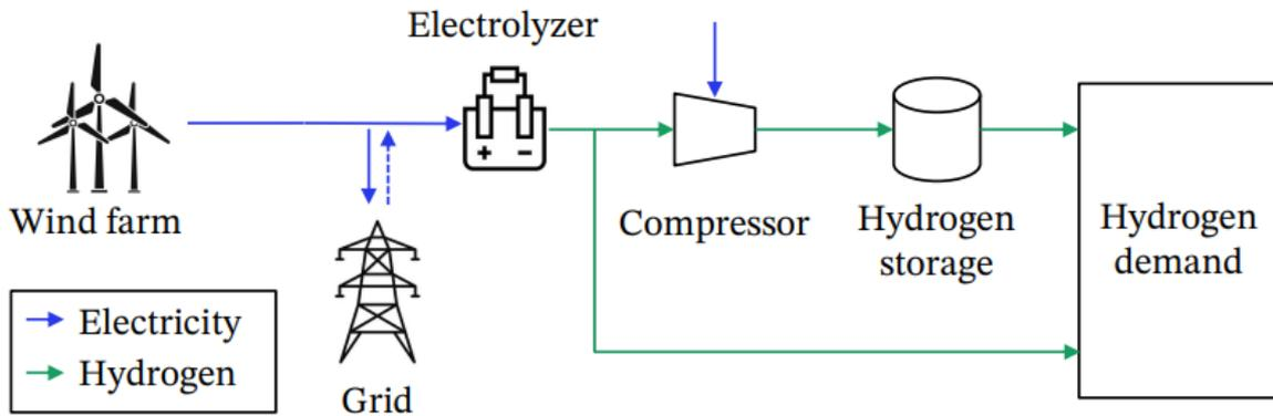
Figure 4.2: System schematic as presented in Baumhof et al. [15]
