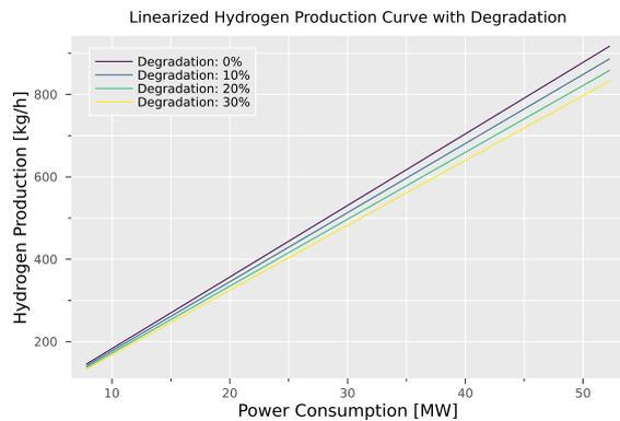
**Figure 4.12:** Effect of degradation on the hydrogen production curve
