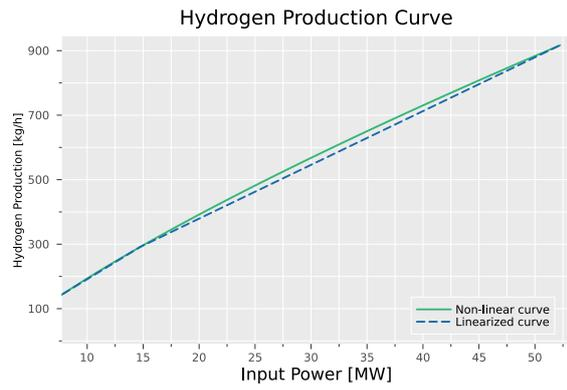
**Figure 4.7:** Non-linear hydrogen production curve with linearized production curve
