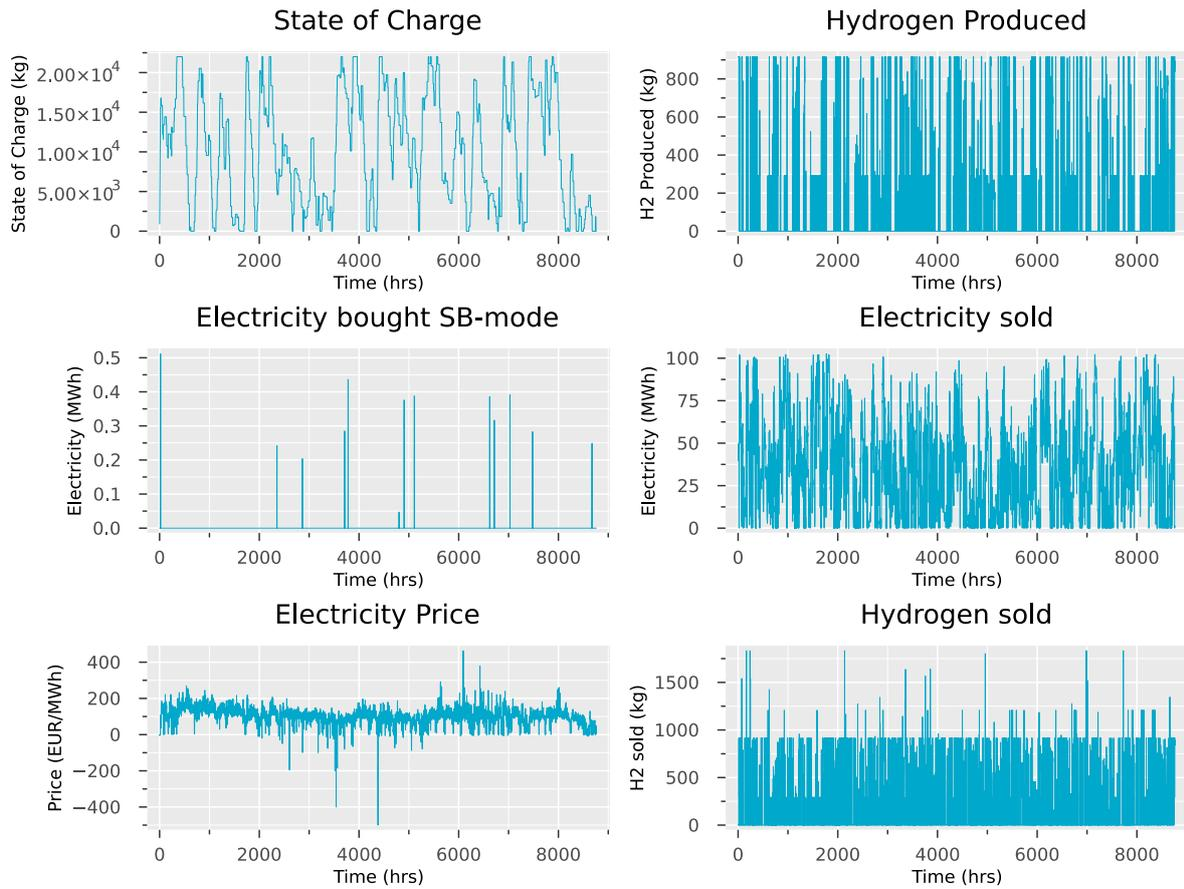
**Figure 5.1:** Operational results from the one-year simulation. The plots show (from top left to bottom right) the state of charge of hydrogen storage, hydrogen production, electricity bought in SB-mode, electricity sold, electricity price, and hydrogen sold.
