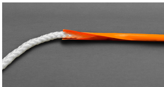
Figure 5. Rope exploration #1 AB plastic protective rope sleeve (in orange) around rope.
