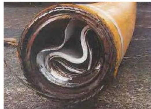
Fig. 3. Collapse failure of the flexible riser [11].
