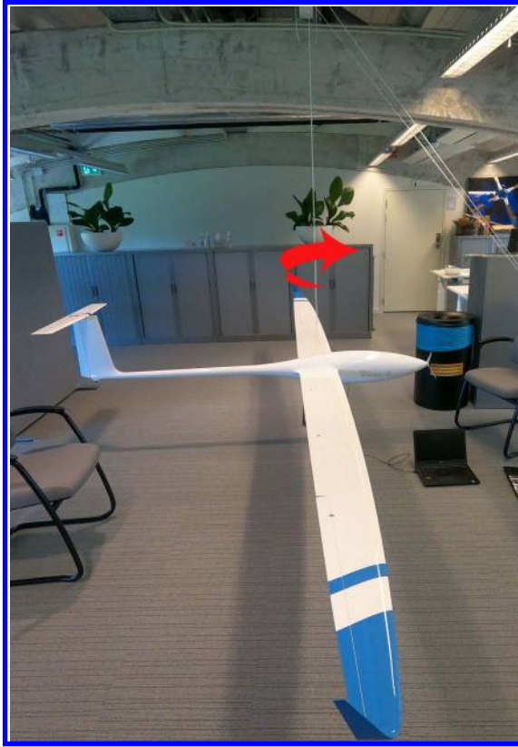
Fig. 4 Yaw moment of inertia setup.
