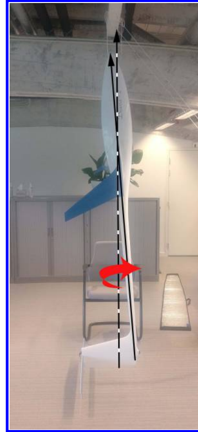
Fig. 5 Roll moment of inertia setup.
