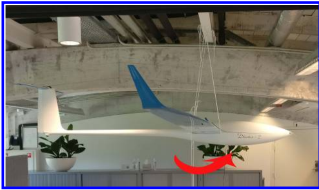
Fig. 2 Pitch moment of inertia setup.
