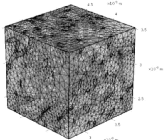
Figure 1. FEM mesh of inTMB reconstructed by CT-scans
