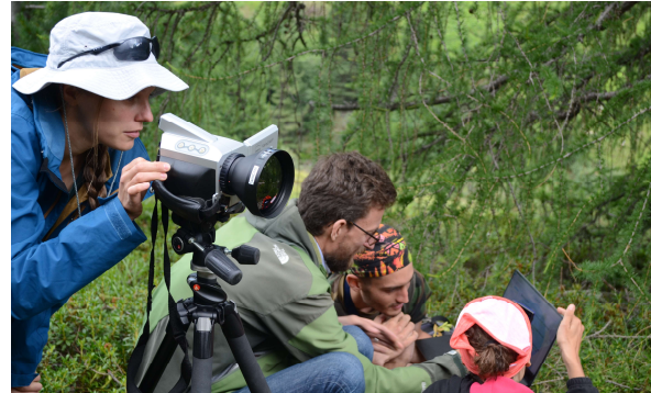
Figure 3. Thermography acquisition in the field
