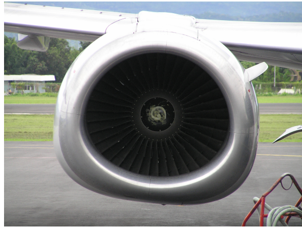
Figure 1.2: The Boeing 737NG features a nacelle with a flattened bottom, which was designed to provide more ground clearance while employing a high BPR engine without the need to redesign the air plane's landing gear and wings.
