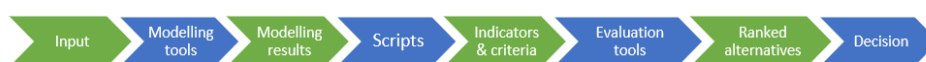
Figure 7.1: Workflow of the NBDSS from input to decision. system components are in blue, input/output in green. The figure shows the relation between output types 1 and 2 and the indicators and criteria.
