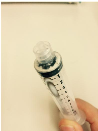
Figure 3.5: Calcium precipitation as observed in TUHDN2C with phosphate
