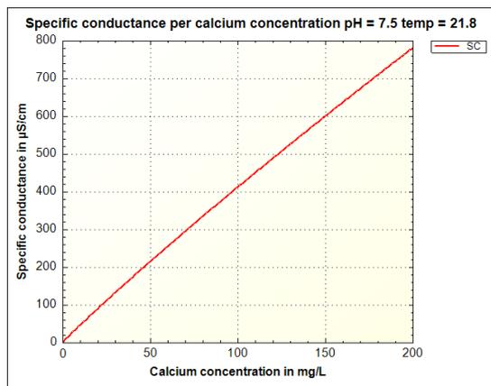
Figure 3.6: Specific conductance per calcium concentration for pH 7 and a temperature of 21.8 degrees Celsius
