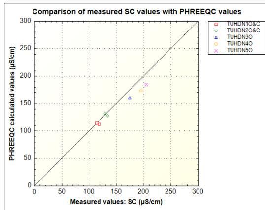
Figure 3.8: SC calculated with PHREEQC compared to measured SC values
