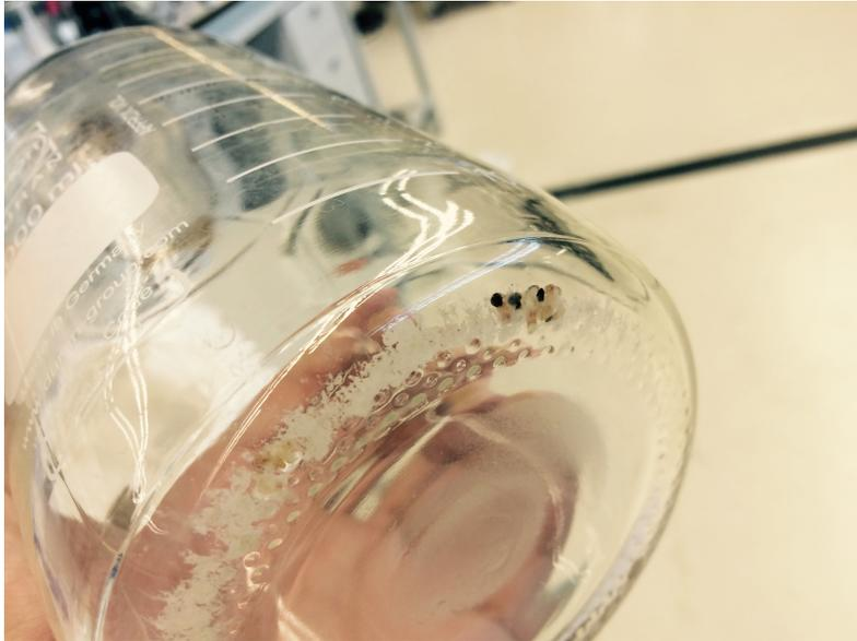
Figure 3.3: Calcium precipitation as observed in TUHDN30 with phosphate
