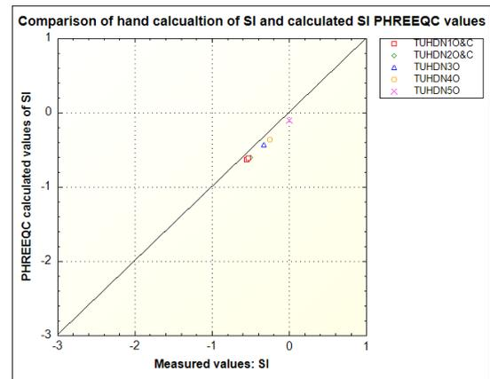
Figure 3.9: SI calculated with PHREEQC compared to measured values
