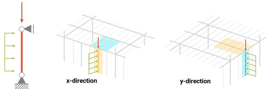
Figure C.6: Facade column pinned at both ends, subjected to vertical loads at the top and horizontal distributed loads along the height
