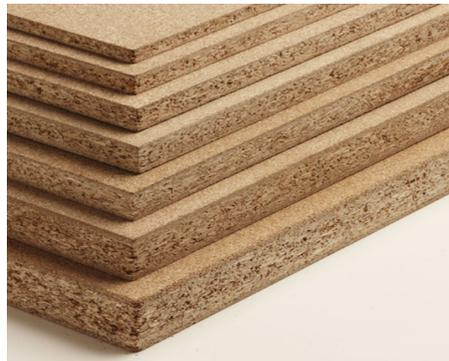
Figure 3.19: Particle boards
