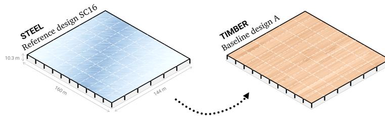
Figure 4.15: timber baseline design A to compared with steel reference design
