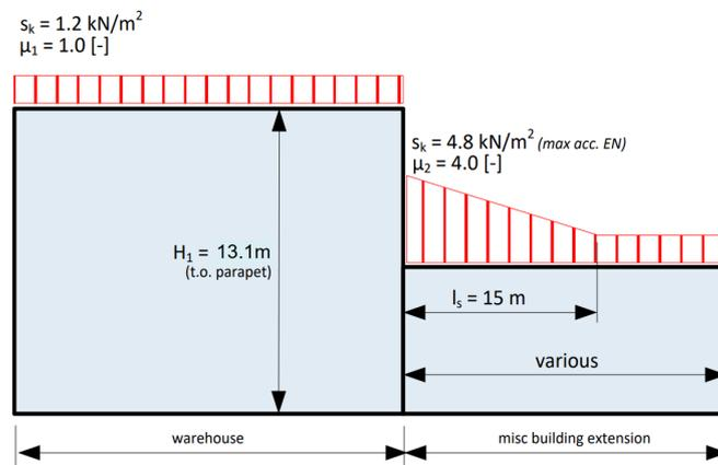
**Figure B.1:** Snow load on the roof of the warehouse (RHDHV Internal Document, 2022)
