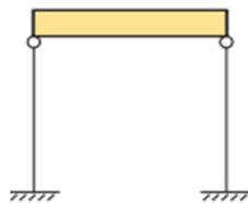
**Figure 4.8:** Stability system of the concrete reference frame: Fixed base columns, hinged roof beams
