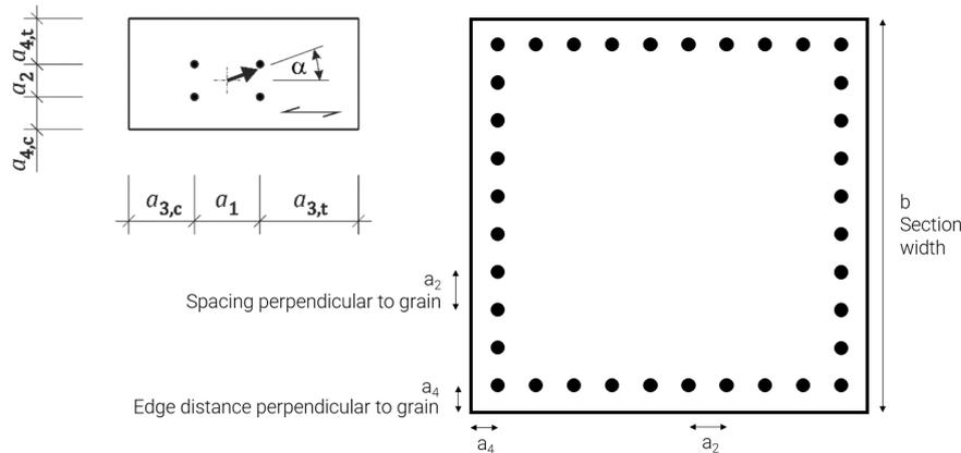
Figure C.10: Glued-in rods layout within the timber section
