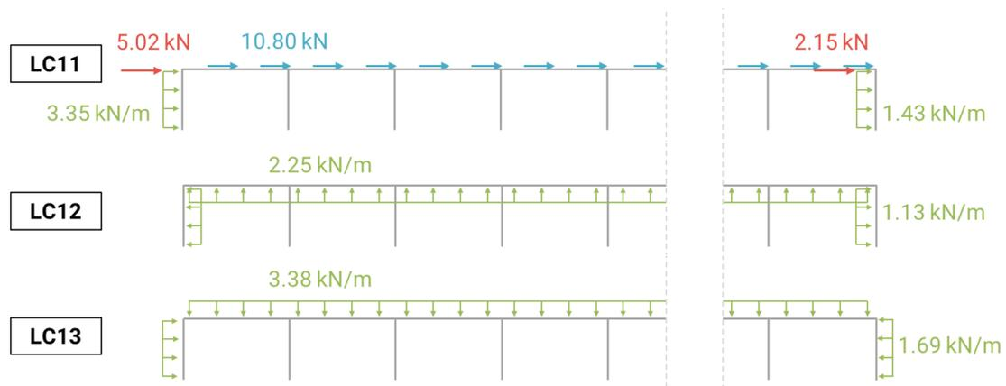
Figure C.4: Overview of loads applied on the 2D warehouse section in the x-direction
