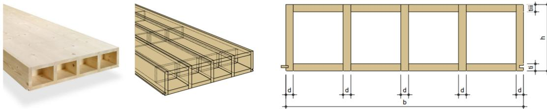
Figure E.6: Dimensions of Lignatur surface element (LFE): height  $h=180\text{mm}$ , width  $b=1000\text{mm}$ , thickness of ribs  $d=31\text{mm}$ , thickness skin  $t_i=31\text{mm}$ , thickness skin  $t_{iii}=31\text{mm}$ , number of boxes  $n=4$ , Length  $L=8\text{m}$ , weight= $38\text{kg/m}^2$  (ETA-11/013, 2021)
