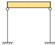
**Figure 4.12:** Stability system of the timber baseline frames: Fixed base columns, hinged roof beams
