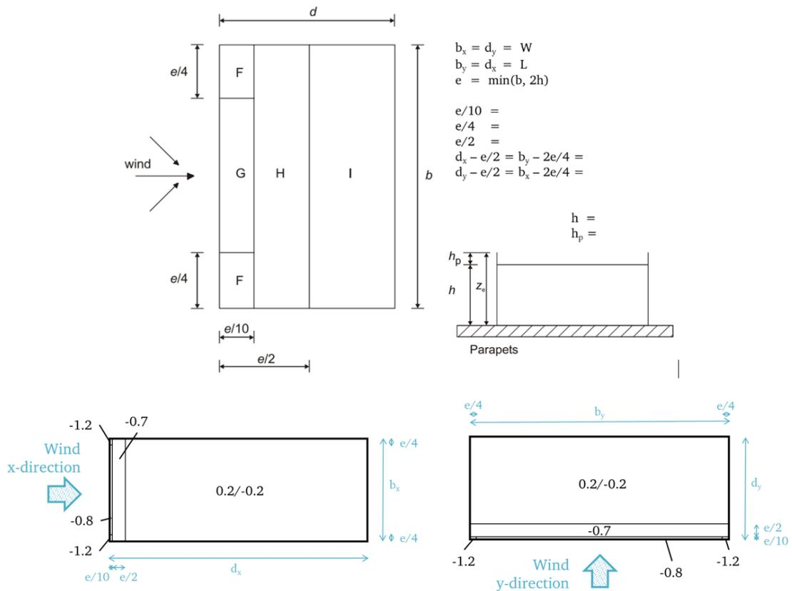
**Figure B.7:** Pressure coefficients  $c_{pe,10}$  for flat roofs with parapets, zones F to I ( $h/h_p=0.1$ ,  $A \geq 10m^2$ ) in accordance with EN 1991-1-4
