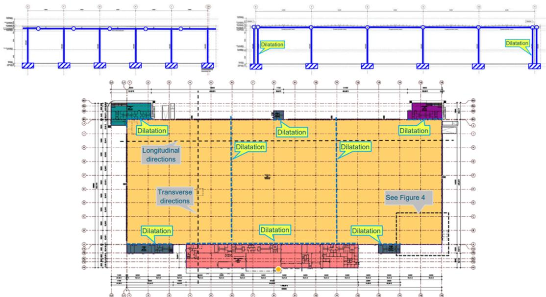
**Figure 4.7:** Typical sections of the concrete (IXD) warehouse with stabilising portal frames in the transverse (top left) and longitudinal (top right) directions, and general layout (bottom) (RHDHV Internal Document, 2020)
