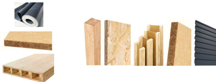
**Figure 5.6:** Biobased envelope build-up: Lignatur panels, wood fibre insulation, EPDM for the roof (left) and glulam mullions, OSB panel, wood I-joists, wood fibre insulation, steel sheathing for the facade (right)
