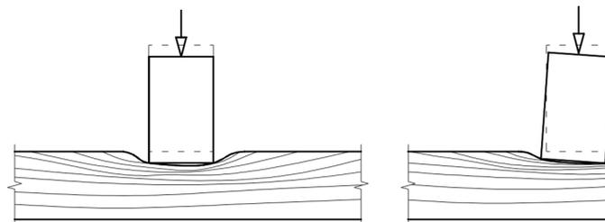
Figure A.4: Bearing effects at supports and points of concentrated load application (NEN-EN 1995-1-1:2005, 2005)
