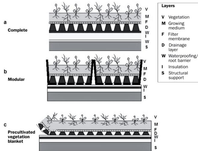
**Figure E.8:** Types of extensive green-roofing technology. (a) Complete systems form integral part of the roof, (b) Modular systems are installed above the existing roof system, (c) Precultivated vegetation blankets are rolled onto the existing roof (Oberndorfer et al., 2007)
