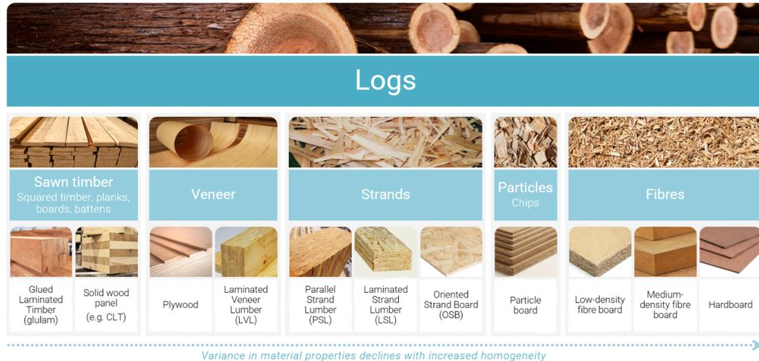
**Figure 3.11:** Types of timber engineered products according to the wood component they are produced from, based on (Blaß & Sandhaas, 2017) and (Sandberg, 2016)
