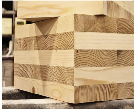
Figure 3.15: Cross Laminated Timber (CLT)
