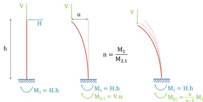
**Figure C.7:** Second order effect increasing bending moments for fixed-based columns subjected to combined gravitational and horizontal loads
