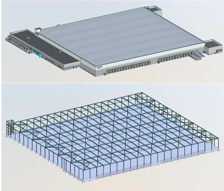
**Figure 4.2:** Steel (SC16) warehouse design overview (top), load-bearing frame, floor slab and foundation pads (bottom)
