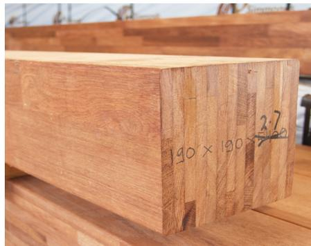
**Figure 3.13:** Glued Laminated Timber (glulam)
