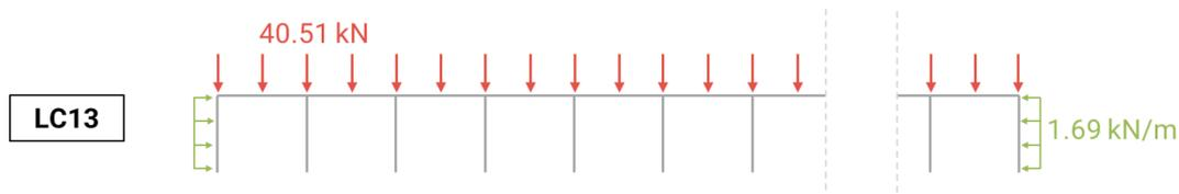
Figure C.5: Overview of loads applied on the 2D warehouse section in the y-direction
