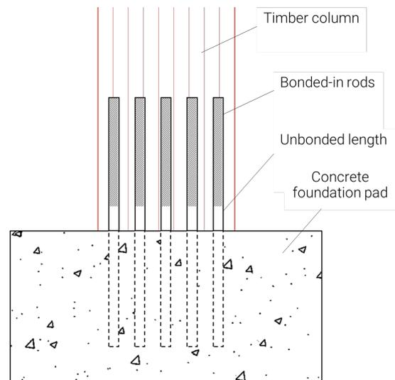
**Figure 4.14:** Detailing of the semi-rigid column base connection in timber baseline designs
