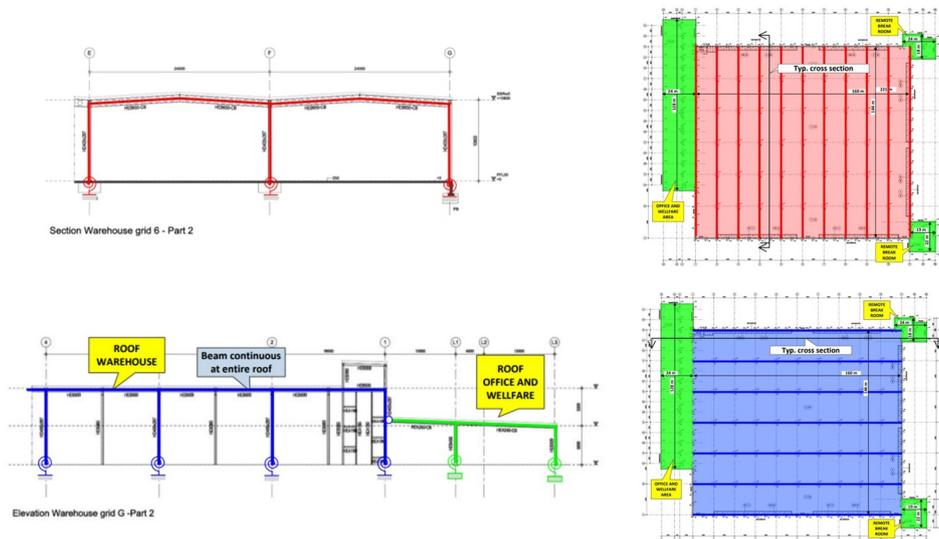
**Figure 4.3:** Typical sections of the steel (SC16) warehouse with stabilising portal frames in the transverse direction (red) and in the longitudinal direction (blue) (RHDHV Internal Document, 2022)
