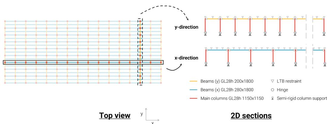
**Figure D.1:** Mechanics scheme of the stabilising frames in the x and y-directions for timber baseline B. Columns and beams are pinned in both directions, the base connection stiffness is 201 MNm/rad (see Section D.3).
