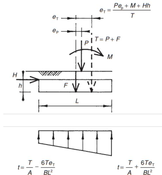
Figure C.12: Capacity check for foundation pads (Curtin et al., 2006)
