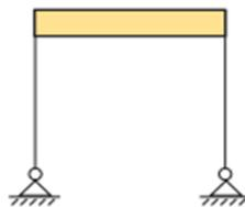
**Figure 4.4:** Stability system of the steel reference frame: Moment fixed connections between columns and roof beams, hinged at the base
