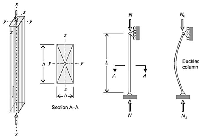
Figure A.7: Buckling of a column (Porteous & Kermani, 2013)
