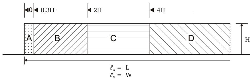
**Figure B.9:** Loading zones of parapets in accordance with EN 1991-1-4
