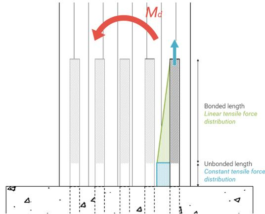
Figure C.13: Glued-in rods connection rotational stiffness calculation model
