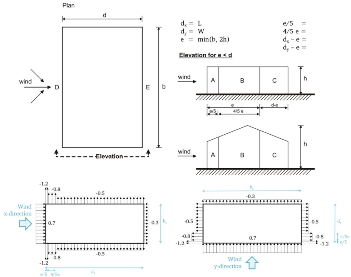
**Figure B.6:** Pressure coefficients  $c_{pe,10}$  for vertical walls, zones A to E ( $h/d \leq 0.25$ ,  $A \geq 10m^2$ ) in accordance with EN 1991-1-4
