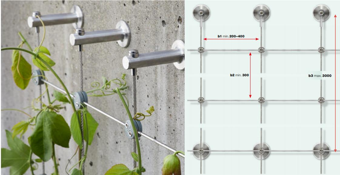
Figure E.9: Indirect greening system and supports dimensions (Jakob Rope Systems, 2020)
