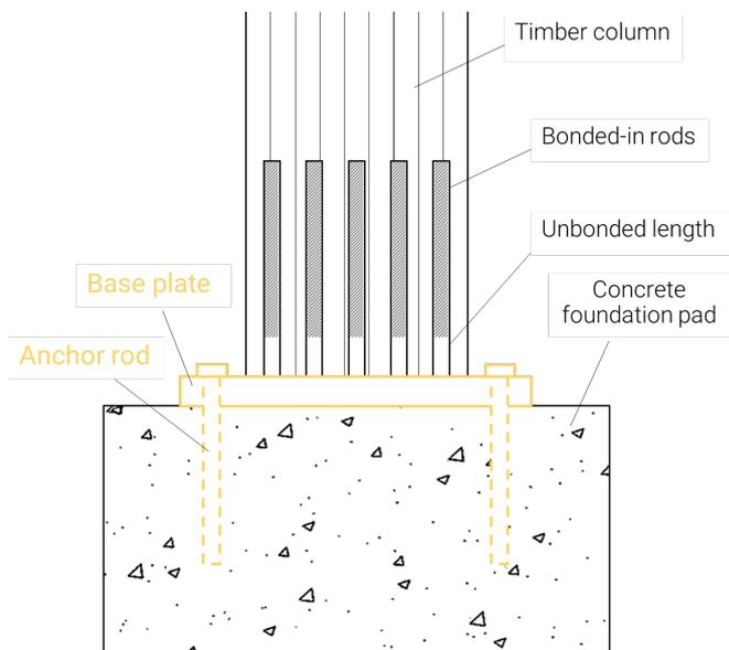
Figure 5.11: Detailing of a demountable glued-in rods connection
