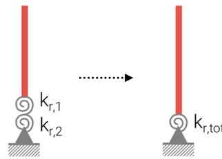
**Figure C.14:** Total rotational stiffness of the base connection
