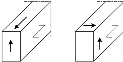
**Figure A.5:** Left: Member with a shear stress component parallel to the grain. Right: Member with both stress components perpendicular to the grain (rolling shear) (NEN-EN 1995-1-1:2005, 2005)
