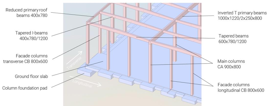
**Figure 4.9:** 3D view of structural elements within the concrete (IXD) warehouse frame (RHDHV Internal Document, 2020)
