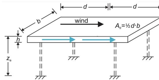
**Figure B.8:** Reference area from friction divided over two points along the length of roof beams, in accordance with EN 1991-1-4
