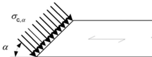
**Figure A.6:** Compressive stresses at an angle to the grain (NEN-EN 1995-1-1:2005, 2005)
