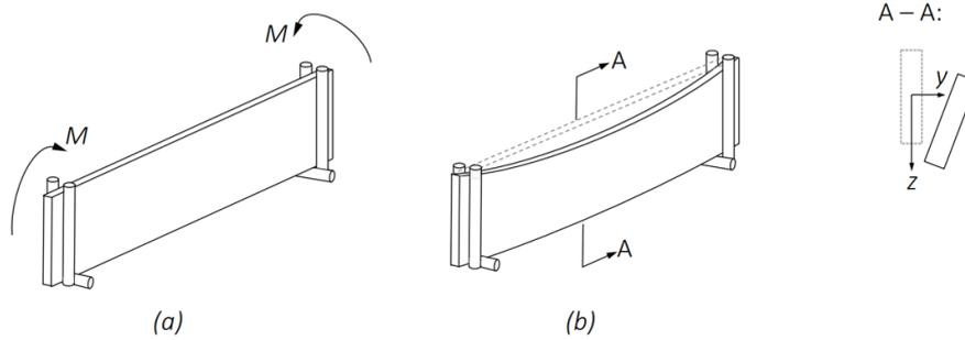
**Figure A.9:** Lateral torsional buckling of a simply supported beam subject to constant moment. (a) simply supported beam with restrained supports, (b) buckled beam (Blaß & Sandhaas, 2017)
