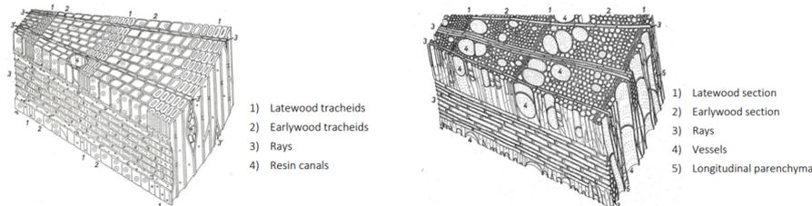
**Figure 3.10:** Schematic structure and cell types of softwood (left) and hardwood (right), Nardi-Berti, 1993 cited by (Blaß & Sandhaas, 2017)
