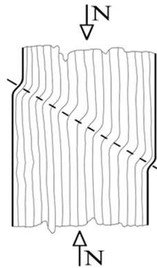
Figure A.3: Failure mechanisms in compression (NEN-EN 1995-1-1:2005, 2005)
