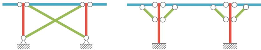
**Figure 5.14:** Diagonal elements (left) and knee bracings (right) to improve lateral stability of the frame
