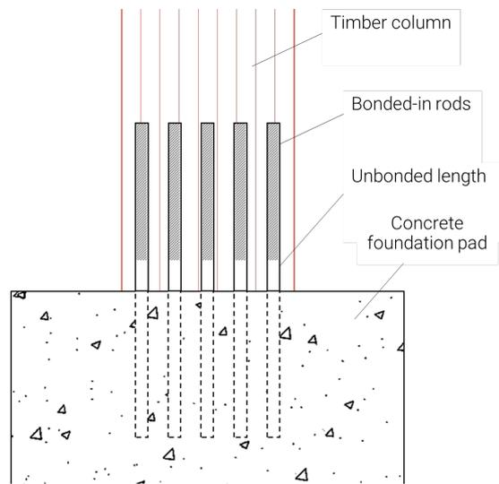
Figure C.8: Main components of the glued-in rods connection
