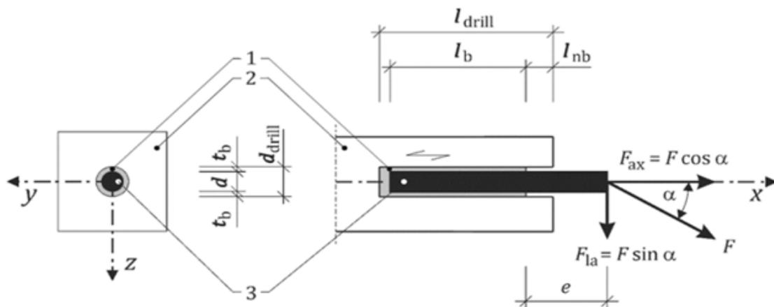
Figure C.9: Geometrical characteristics of glued-in rods
