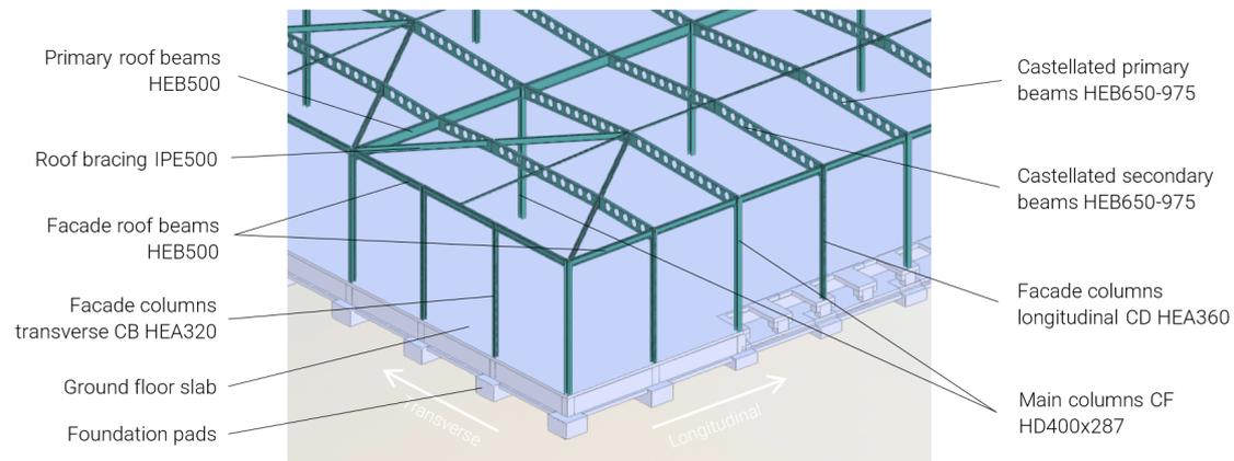
**Figure 4.5:** 3D view of structural elements within the steel (SC16) warehouse frame (RHDHV Internal Document, 2022)
