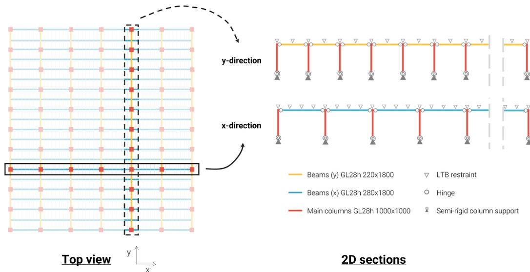
**Figure C.2:** Mechanics scheme of the stabilising frames in the x and y-directions for timber baseline A. Columns and beams are connected by pinned connections in both directions, the stiffness of the column base connection is 110 MNm/rad as calculated in Section C.5.
