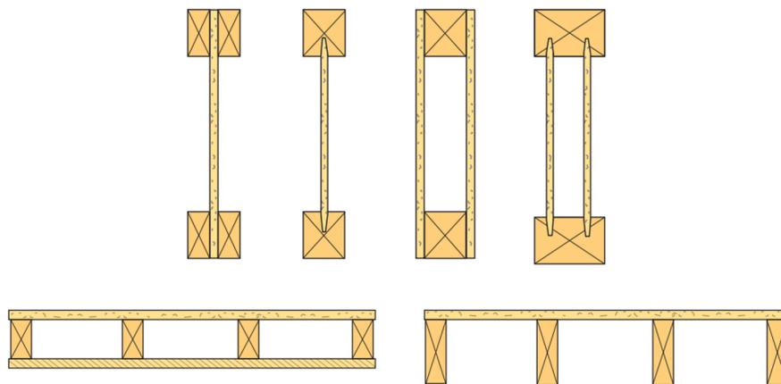
**Figure 3.20:** Typical cross-sections of thin webbed beams and stressed skin panels: I-sections and box-sections (top), H and T sections (bottom) (Norlin, 2016)
