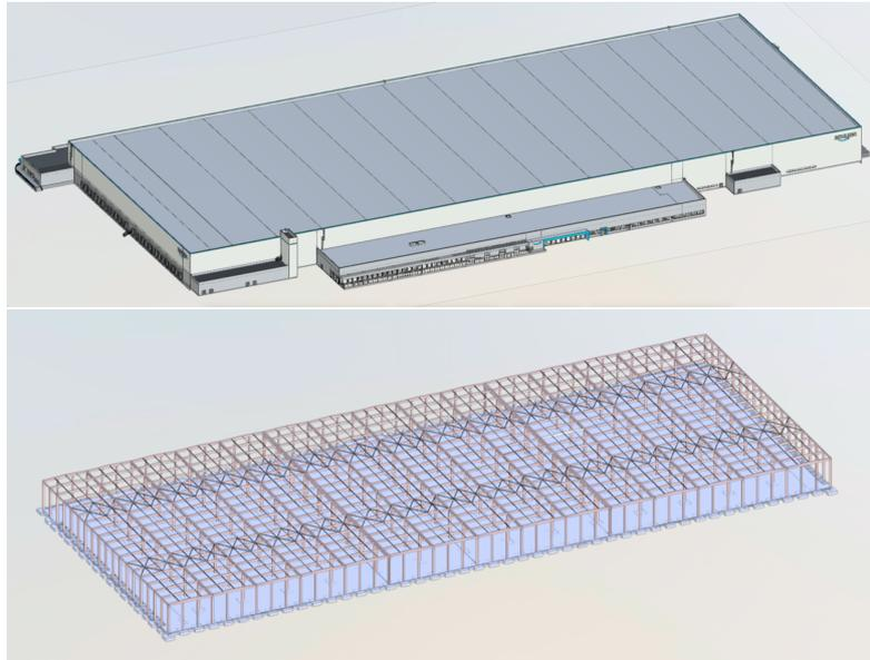
**Figure 4.6:** Concrete (IXD) warehouse design overview (top), load-bearing frame, floor slab and foundation pads (bottom)
