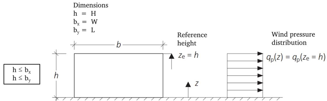
**Figure B.4:** Reference height  $z_e$  depending on  $h$  and  $b$  and wind pressure distribution (NEN-EN 1991-1-4:2005, 2005)
