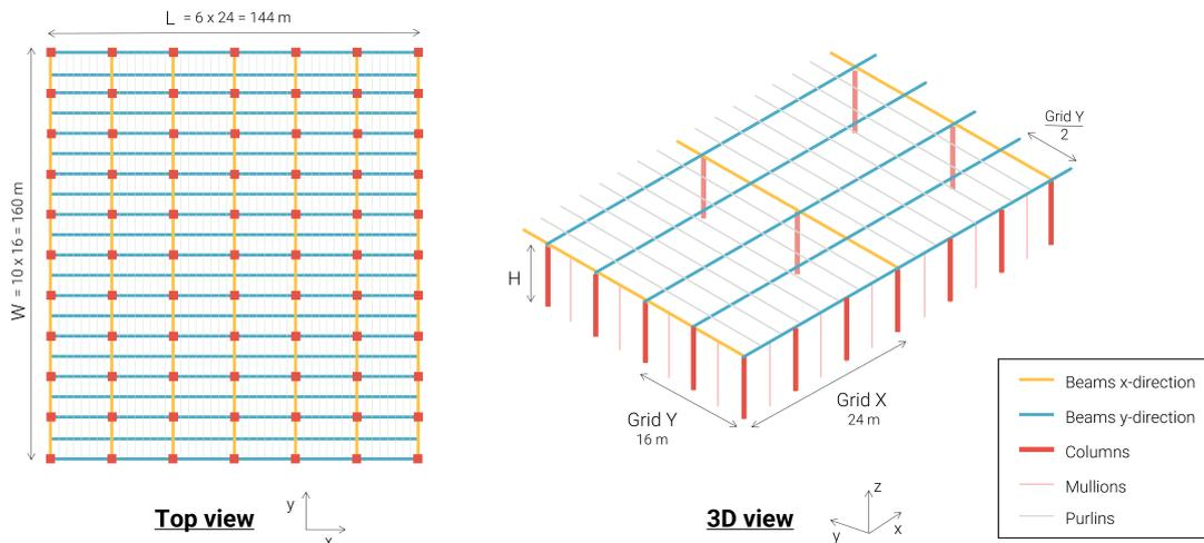
Figure 4.11: Top and 3D view of the timber baseline A load-bearing frame
