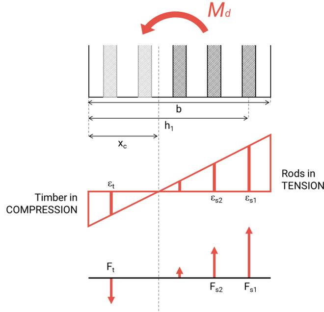
**Figure C.11:** Principle of moment capacity calculation for a glued-in rods connection, strain/forces diagram
