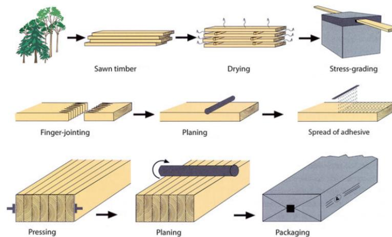
**Figure 3.14:** Manufacturing process of Glued Laminated Timber (Sandberg, 2016)
