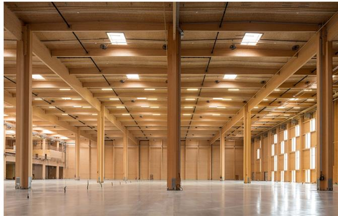
Figure 5.13: Ilogistics Center (Fischamend, Austria) with cruciform glulam columns
