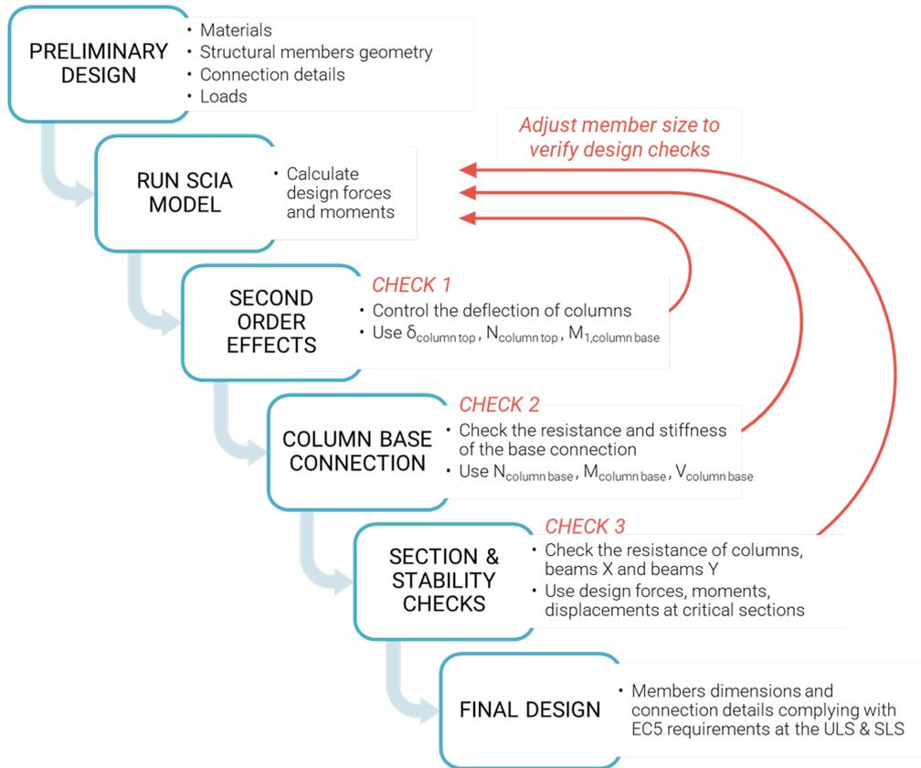
**Figure C.1:** Overview of the structural design process
