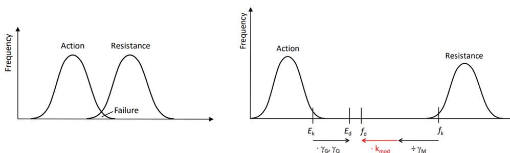
**Figure A.1:** Frequency distributions for action and resistance (left) and reduction of the probability of failure through partial safety factors and  $k_{mod}$  (right) (Blaß & Sandhaas, 2017)
