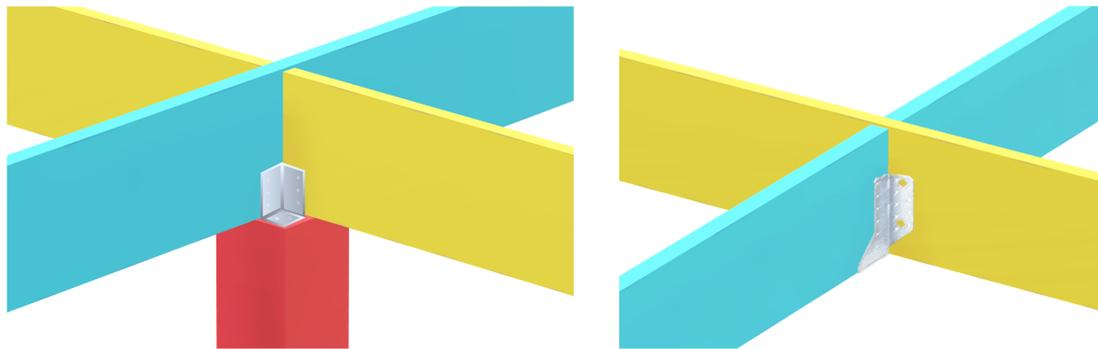
**Figure 4.13:** Detailing of the hinged top connections in timber baseline designs
