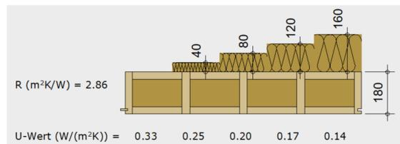
**Figure E.7:** Wood fibre thermal insulation in Lignatur surface element (LFE) - The heat conductivity of coniferous wood is taken as  $\lambda=0.130\text{ W}/\text{mK}$ , and for wood fibre  $\lambda=0.040\text{ W}/\text{mK}$ .
