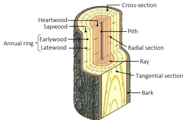
Figure 3.8: Macroscopic structure and section planes of wood (Blaß & Sandhaas, 2017)
