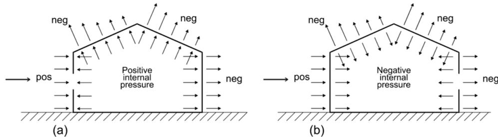
**Figure B.10:** Definition of positive and negative internal wind pressures
