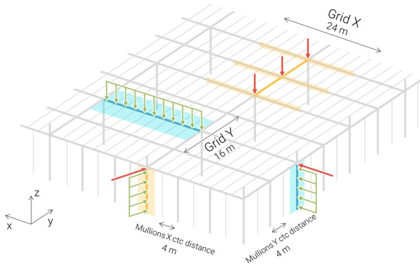
**Figure C.3:** Surface loads on the roof and facades are converted to line loads and point loads in the 2D models. Loads on section (x) are represented in blue and loads on section Y are represented in yellow
