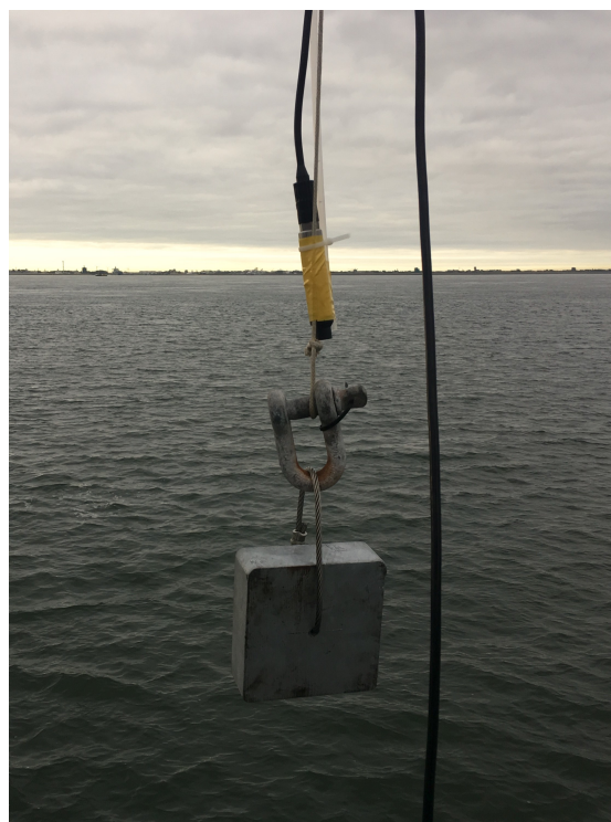
Figure 3.3: Pumping tube and OBS configuration on a pole with the weight on the bottom to keep the measurements in place.
