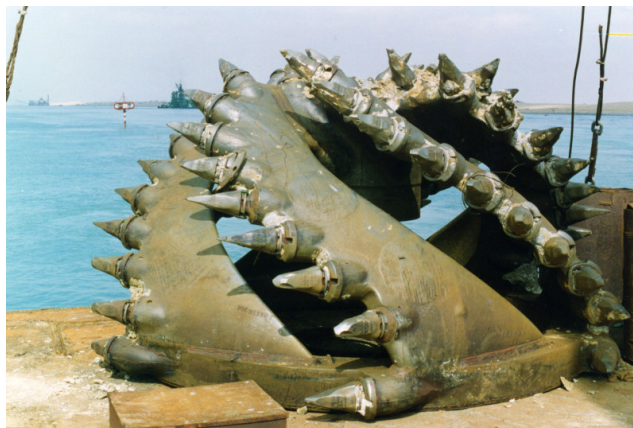
Figure 1.1: Wear on dredge cutter [2]
