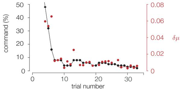
Fig. 5. Typical 3-down/1-up adaptive staircase procedure. The desired friction modulation amplitude is plotted in black and the resulting friction variation amplitude  $\delta\mu$  is plotted in red. The red line reports the mean value of the last six trials.
