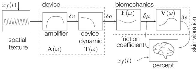
Fig. 2. The signal is generated from a lookup table indexed as a function of the user's position  $x_f(t)$ . The signal is then amplified and the voltage modulation  $\delta v$  is sent to the piezoelectric actuators. Changes in the ultrasonic vibrations of the plate  $\delta a$  result in changes in the frictional force  $\delta \mu$ , which creates skin vibrations, captured by an accelerometer on the skin surface on the first phalanx of the finger  $\delta s$ .
