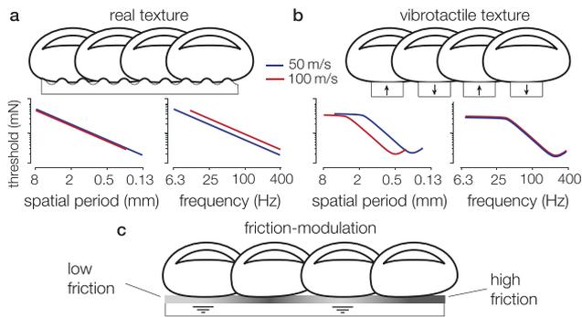
Fig. 1. **a.** Detection threshold curve with a spatially based perception model in the spatial and frequency domains. Data extracted from [8], [9]. **b.** Detection threshold curve with a frequency based perception model in the spatial and frequency domains. Data extracted from [6]. 50 mm/s and 100 mm/s velocities are shown in blue and red respectively. **c.** Interaction with a virtual texture on a surface-haptic device.
