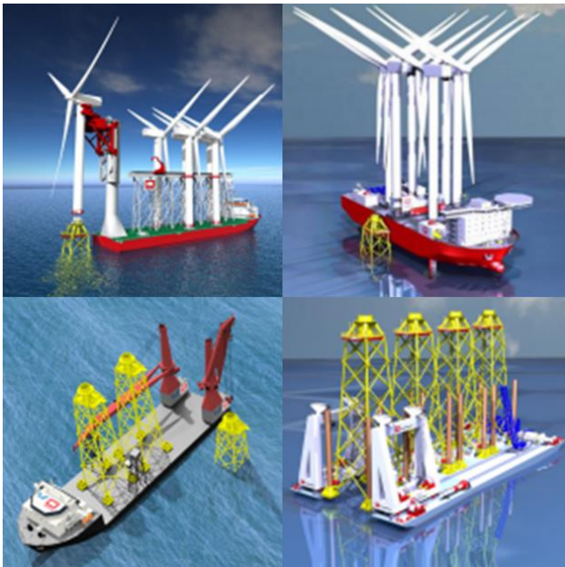
Figure 25 Wind turbine installation concept vessels (Harst, 2013, slide 6)
