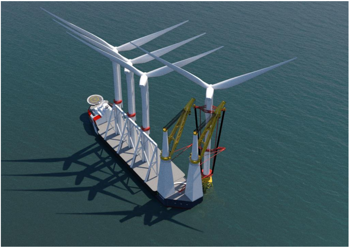
Figure 115 Detailed 3D model of PWT installation concept ©Marc Brinkman
