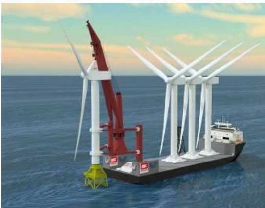
Figure 24 Single lift wind turbine installation with stabilization arms (Horst, 2011, slide 16)
