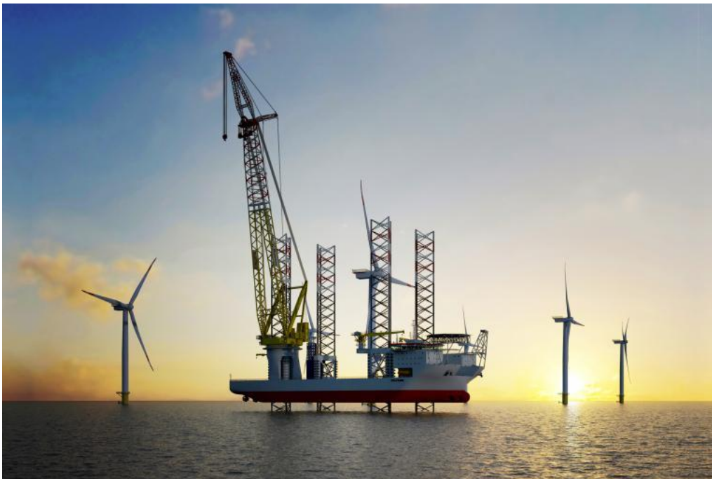
Figure 18 New generation jack-up vessel Voltaire of Jan de Nul (Jan de Nul, n.d.)
