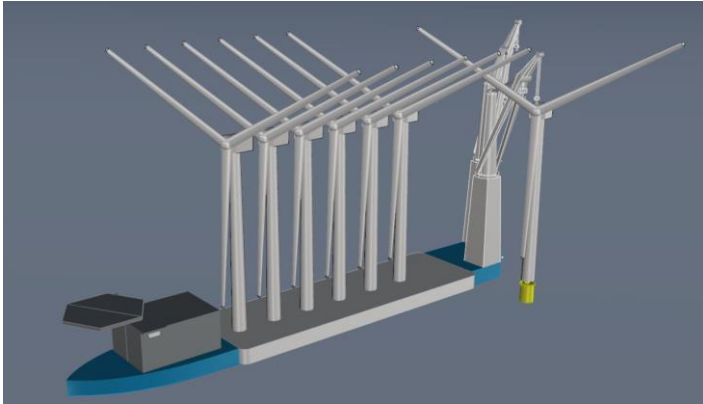
Figure 110 Application small wind turbine installation with single crane
