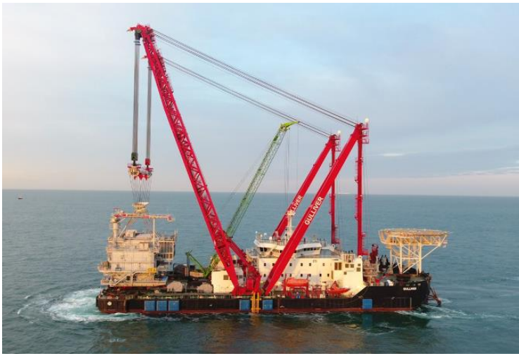
Figure 53 Gulliver transporting offshore substation (Scaldis, 2020)
