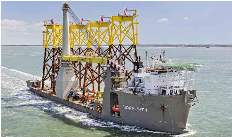
Figure 11 Bokalift 1 of Boskalis transporting jackets (Boskalis, n.d.)
