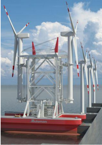
Figure 23 Wind Turbine Shuttle of Huisman (Huisman, n.d.a)
