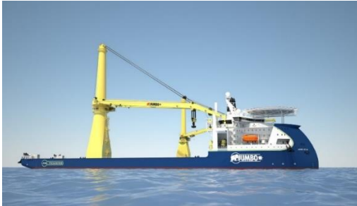
Figure 83 Jumbo Stella Energy with offshore mast crane (Ulstein, 2017)
