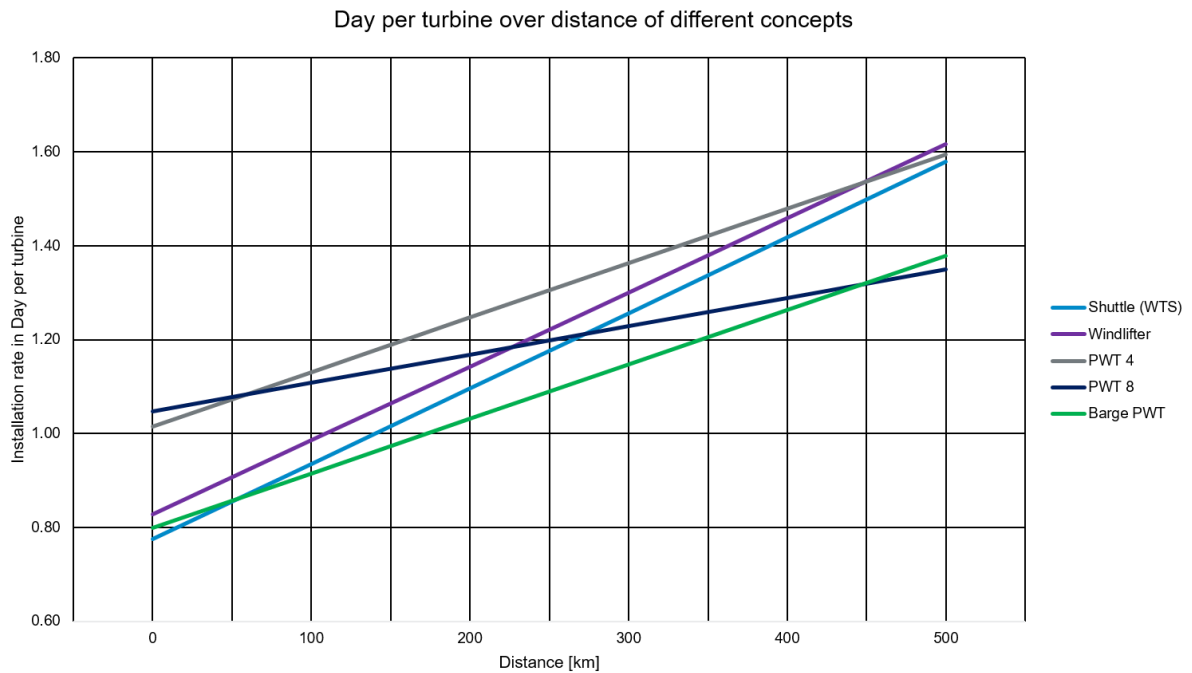
Figure 74 Installation rate (Day per turbine) over distance for promising concepts
