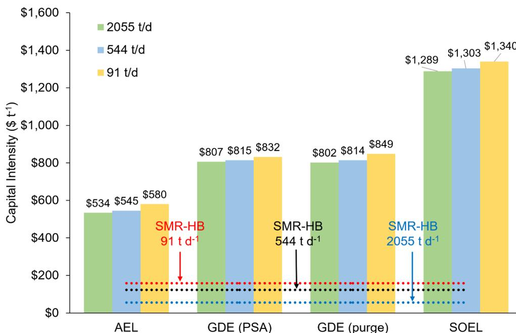
**Figure 4.2:** Capital intensity ( $\$ t^{-1}$ ) of different electrolyzer configurations. SMR-HB capital intensity data is based on the forthcoming publication by Izelaar et al. [31].
