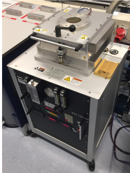
Figure 3.8: Reflow oven SRO702/704 used in sample preparation
