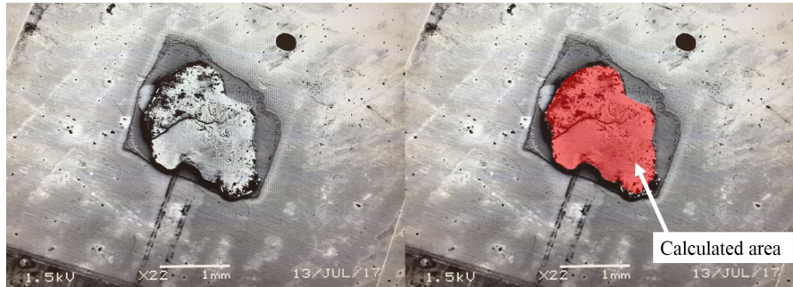
Figure 3.17: Au-Sn solder joint area measurement by counting pixels from SEM images
