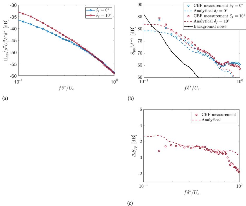
Figure A.6: Wall-pressure spectrum measured by the first pressure sensor of the trailing edge (M09) compared against PIV data and analytical models. Measurements are given at  $\delta_f = 0^\circ$  (a) and  $\delta_f = 10^\circ$  (suction and pressure side, b, and c respectively). Measured and estimated changes in the pressure spectrum with respect to the  $\delta_f = 0^\circ$  case are presented in (e) and (f).
