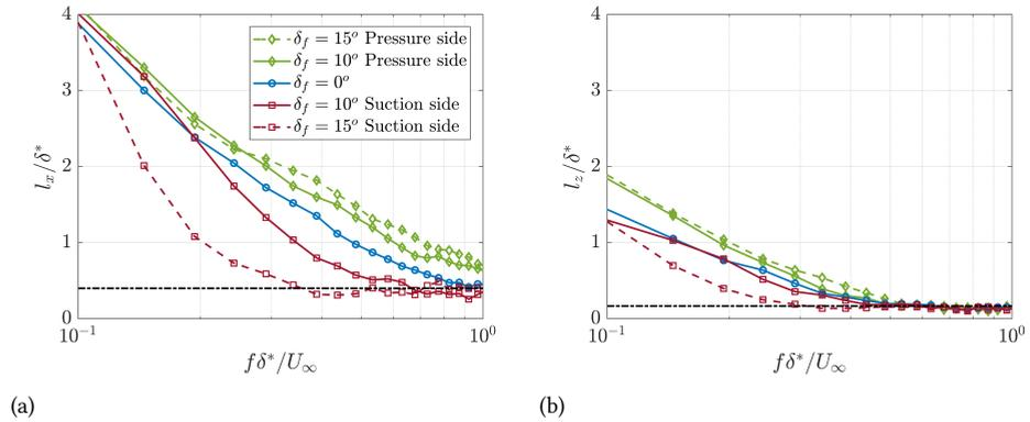
Figure 5.7: Measured streamwise and spanwise correlation length along the trailing-edge serration from the surface microphone sensors at  $\delta_f = 0^\circ$ ,  $10^\circ$  and  $15^\circ$ . The black dot-dashed lines represent the limit of the measurement technique considering coherence levels below 0.05 for two adjacent microphone sensors.
