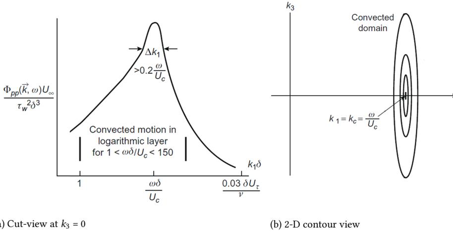
Figure 2.7: Representation of the shape of the frequency-filtered two-wavenumber spectrum of the compressible wall-pressure fluctuations beneath a turbulent boundary layer. Figure adapted from the work of [42].
