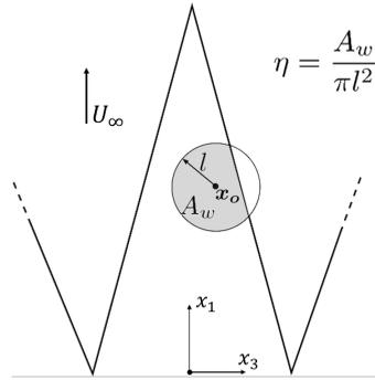
Figure 6.2: Representative view of the radius of influence of the wall-bounded region in a point  $\mathbf{x}_o = (x_{1,o}, x_{3,o})$  and the procedure applied to compute the factor  $\eta$  over a serrated trailing-edge.
