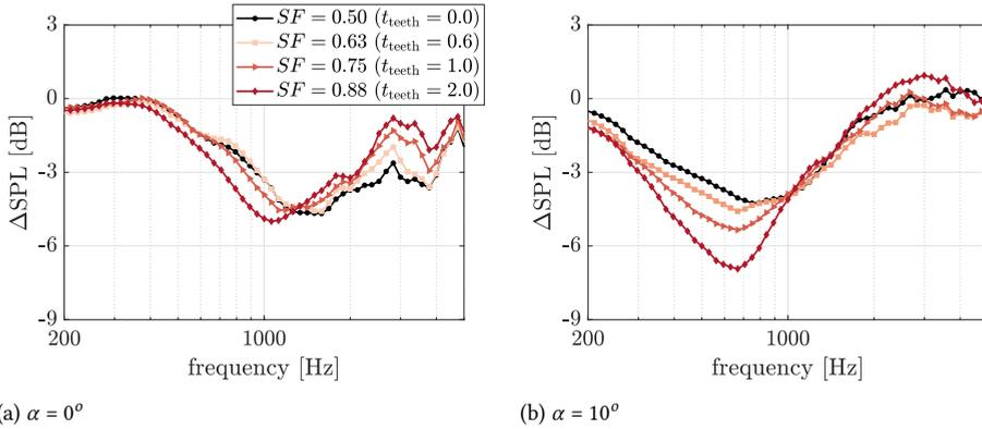
Figure 7.11: Measured noise reduction ( $\Delta SPL$ ) obtained at  $U_\infty = 30$  m/s by varying the solidity factor ( $SF$ ) of the combs in the combed sawtooth design. (a)  $\alpha = 0^\circ$ , and (b)  $\alpha = 10^\circ$ .
