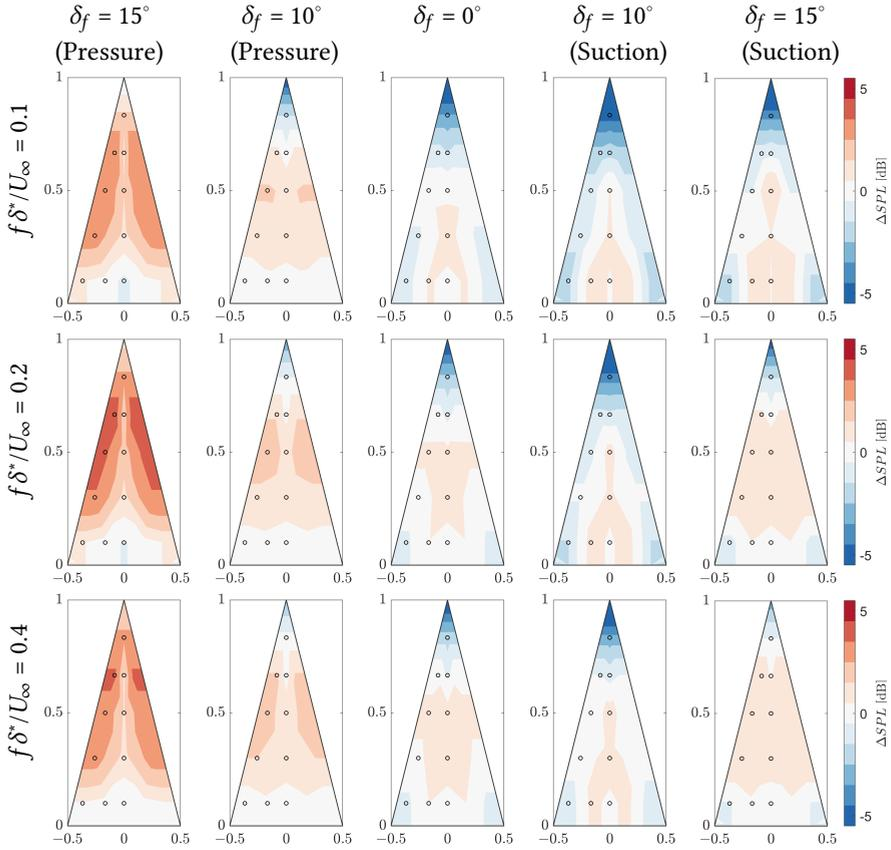
Figure 5.4: Surface pressure fluctuations along the trailing-edge serration relative to the incoming level (reference Mic 09). Trailing-edge incidence angle  $\delta_f$  varies along columns. Strouhal number varies across rows. The circles represent the position of the sensors.
