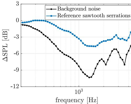
Figure 4.15: Measured difference between background noise and baseline noise levels (black curve) obtained with source power integration from the centre span region. The difference between the reference sawtooth serration design and the baseline noise levels is shown in blue. Negative values of  $\Delta\text{SPL}$  indicate noise reduction. Background noise measurements are obtained by removing the model from the test section while measuring at the same flow speed.
