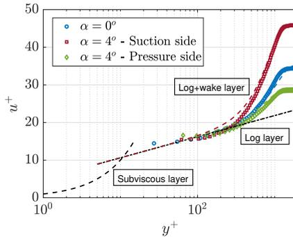
Figure 5.15: Boundary-layer profile near the trailing edge for the baseline case at  $\alpha = 0^\circ$  (a), and  $\alpha = 4^\circ$  ( $Re = 2,000,000$ ). Linear, logarithmic and logarithmic + wake laws are plotted.
