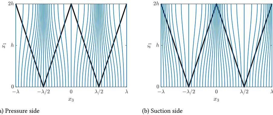
Figure 6.3: Illustrative streamlines of the flow created by the superposition of a Taylor-Green vortex with wavenumbers defined as  $\bar{k}_1 = \pi/2h$  and  $\bar{k}_3 = 2\pi/\lambda$  to the uniform flow.
