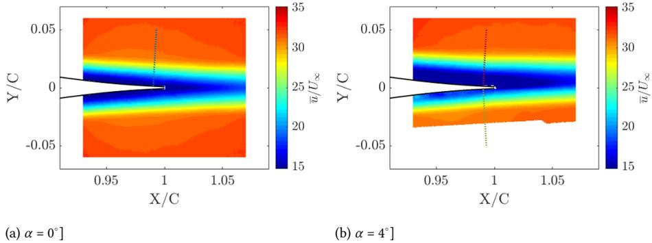
Figure 5.14: Flow field near the trailing edge for the baseline case at  $\alpha = 0^\circ$  (a), and  $\alpha = 4^\circ$  ( $Re = 2,000,000$ ). Wall normal lines denotes the region where the boundary-layer profile was extracted.
