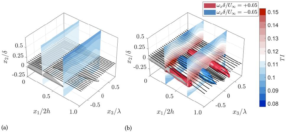
Figure 5.3: Spatial distribution of turbulence intensity (TI) at  $\delta_f = 0^\circ$  (a) and  $\delta_f = 10^\circ$  (b) by cross-sections at  $x_1/2h = 0.25$  and  $0.75$ . Isosurfaces of streamwise vorticity as from Figure 5.2. Black lines show the streamlines of the flow at 8 mm from the wall.
