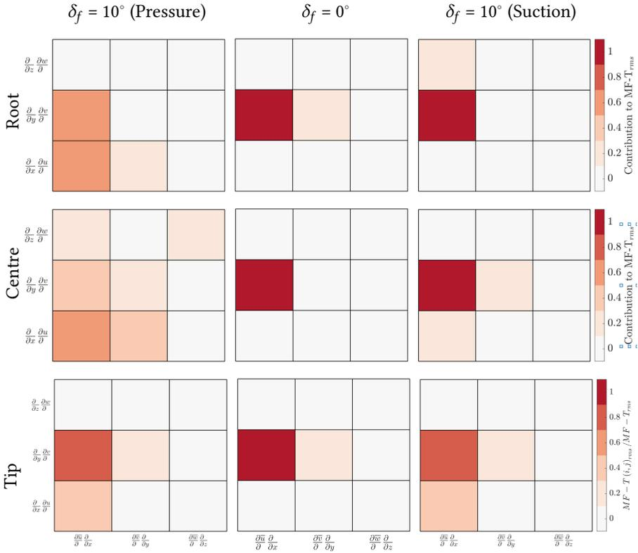
Figure 5.10: Relative contribution of the root-mean-squared of each component  $\frac{\partial \overline{U}_i}{\partial x_j} \frac{\partial u_j}{\partial x_i}$  to the mean shear-turbulence (MS-T) interaction term of the pressure Poisson equation estimated along the edges of the serration (one momentum thickness above the wall). Different flap angles,  $\delta_f = 0^\circ$  (b, e, and h) and  $\delta_f = 10^\circ$  on the pressure (a, d, and g) and suction sides (c, f, and i) are represented.
