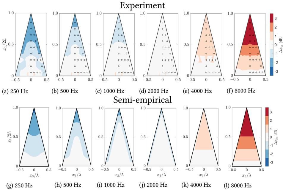
Figure 6.8: Distribution of the wall-pressure fluctuations over the serration surface for  $\alpha = 0^\circ$  and  $Re = 2 \times 10^6$ . Reference is set to the sensor at the centre root of the serration. Figures (a) to (f) show the measured wall-pressure levels and figures (g) to (l) show the predicted distributions.
