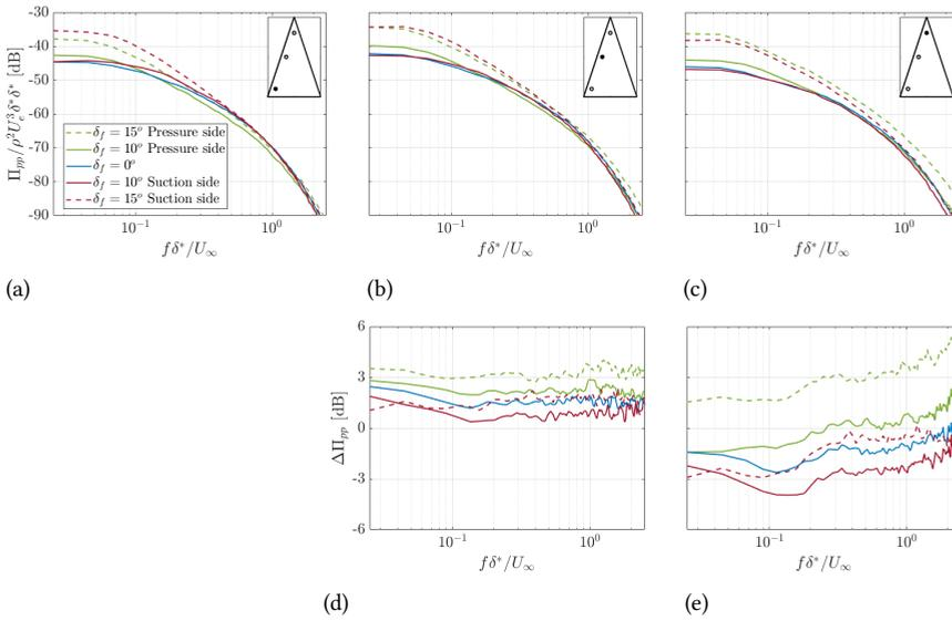
Figure 5.8: Variation of the scattering energy spectrum along the serration edge and relative change in relation to the root ( $x_1/2h = 0.1$ ), at  $x_1/2h = 0.1$  (a),  $x_1/2h = 0.5$  (b and d), and  $x_1/2h = 0.8$  (c and e).
