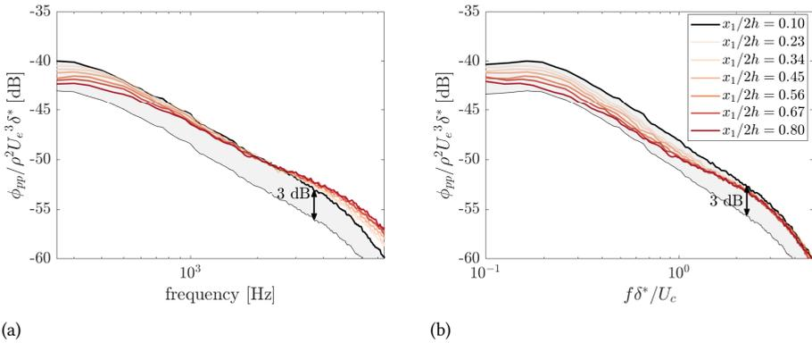
Figure 6.7: Measurements of the wall-pressure spectrum along the centre of the serration for  $\alpha = 0^\circ$  and  $Re = 2 \times 10^6$ . Figure (a) shows the wall-pressure levels with no scaling applied in the frequency and (b) with the frequency scaled with the local convection velocity. The grey area illustrates the maximum possible reduction hypothesized (3 dB) from equation 6.1.
