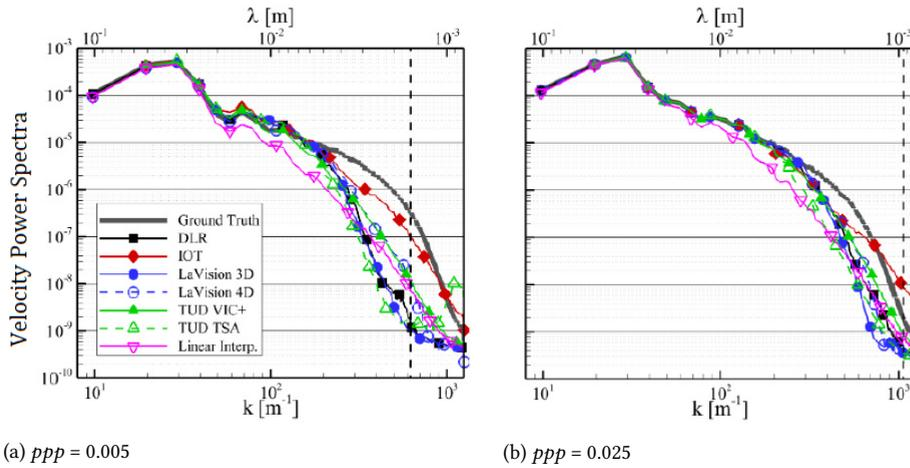
Figure 3.15: Comparison of the wavenumber spectra of the velocity fluctuations obtained from numerical simulation (ground truth), and different data-assimilation techniques. Image from the work of Sciacchitano et al. [104] for different particle concentrations. The dashed line shows the mean distance between particles.
