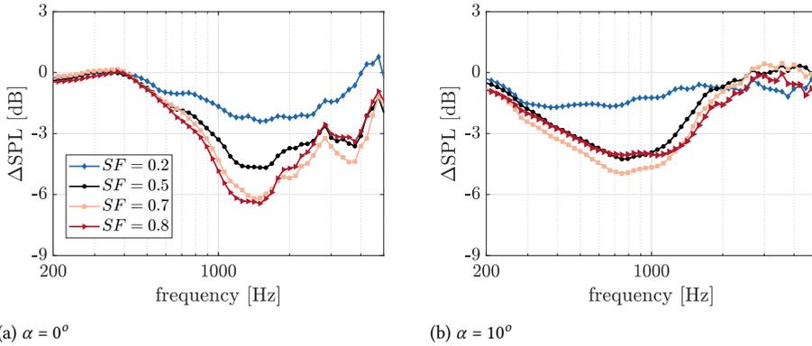
Figure 7.9: Measured noise reduction ( $\Delta SPL$ ) obtained at  $U_\infty = 30$  m/s by varying the serration geometry parameterized with the solidity factor  $SF$ . (a)  $\alpha = 0^\circ$ , and (b)  $\alpha = 10^\circ$ .
