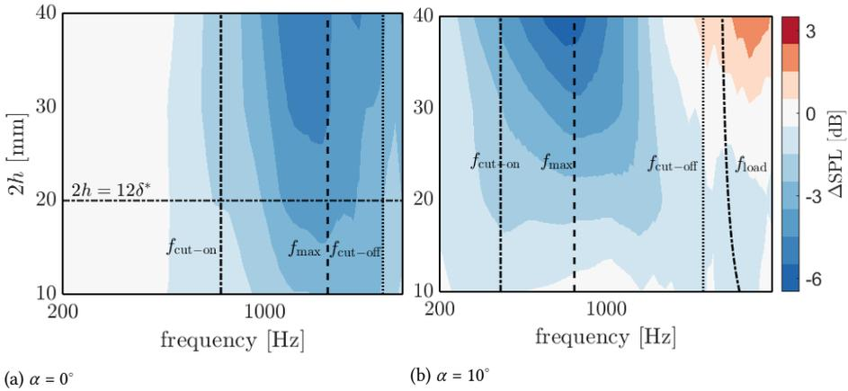
Figure 7.4: Contour plot of the variation of noise reduction for  $\alpha = 0^\circ$  (a), and  $\alpha = 10^\circ$  (b) at  $U_\infty = 30$  m/s with the variation of serration height while the wavelength is kept constant ( $\lambda = 15$  mm). Black lines show the theoretical predictions for the cut-on, max, cut-off, and loading noise frequencies.
