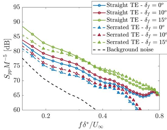
Figure 5.1: Acoustic noise levels estimated from the SPI procedure of the CBF maps. Measurements are performed with a straight and a serrated trailing-edge insert at  $\delta_f = 0^\circ$ ,  $10^\circ$  and  $15^\circ$ .
