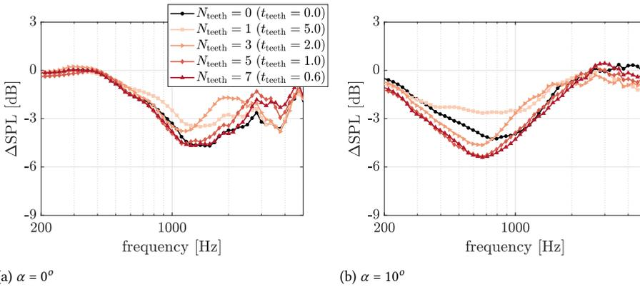
Figure 7.10: Measured noise reduction ( $\Delta SPL$ ) obtained at  $U_\infty = 30$  m/s by varying the number of combs ( $N_{teeth}$ ) in the combed sawtooth design. (a)  $\alpha = 0^\circ$ , and (b)  $\alpha = 10^\circ$ .
