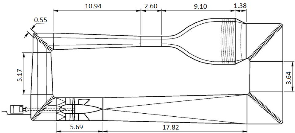
Figure 4.8: Low Turbulence wind Tunnel (LTT) circuit.
