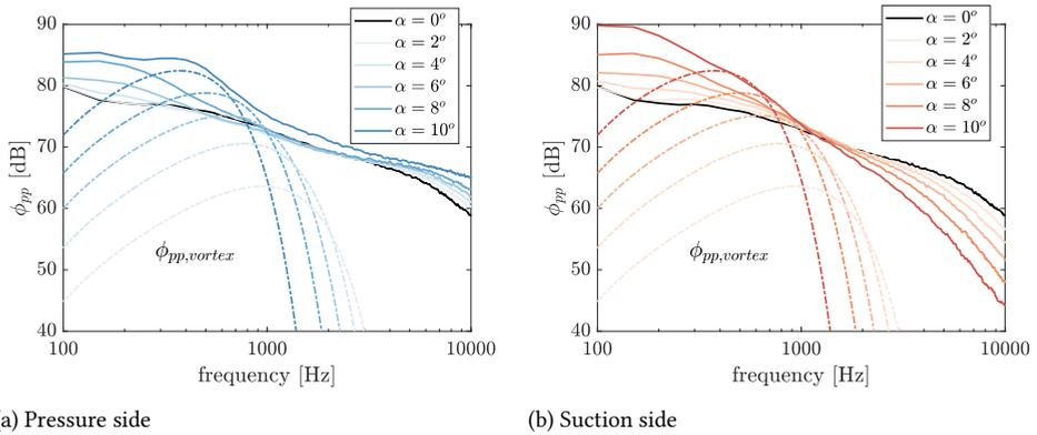
Figure 6.12: Comparison between measured  $\phi_{pp}$  (solid lines) and predicted aerodynamic loading effects (dashed dotted lines) at the sensor located at the serration tip ( $Re = 2 \times 10^6$ ). (a) shows the spectrum on the pressure side and (b) on the suction side.
