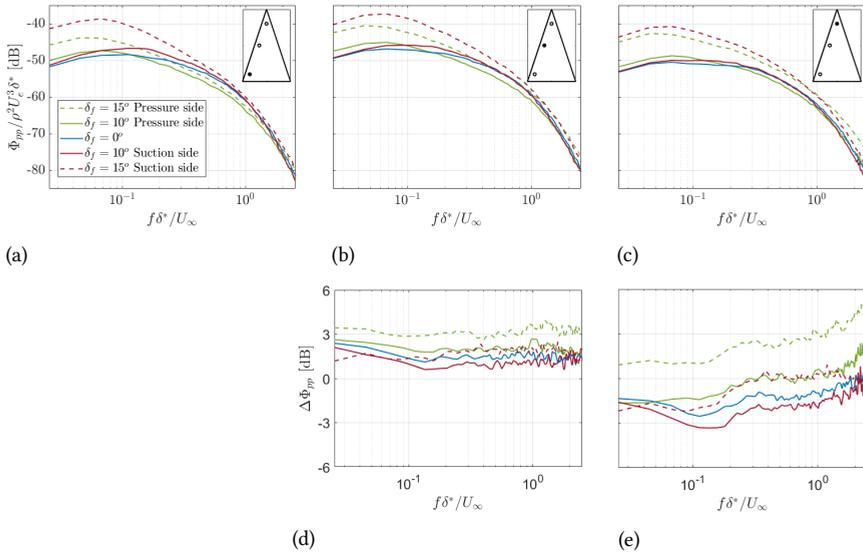
Figure 5.5: Variation of the wall-pressure spectrum along the serration edge and relative change in relation to  $x_1/2h = 0.1$  at  $x_1/2h = 0.1$  (a),  $x_1/2h = 0.5$  (b and d), and  $x_1/2h = 0.8$  (c and e).
