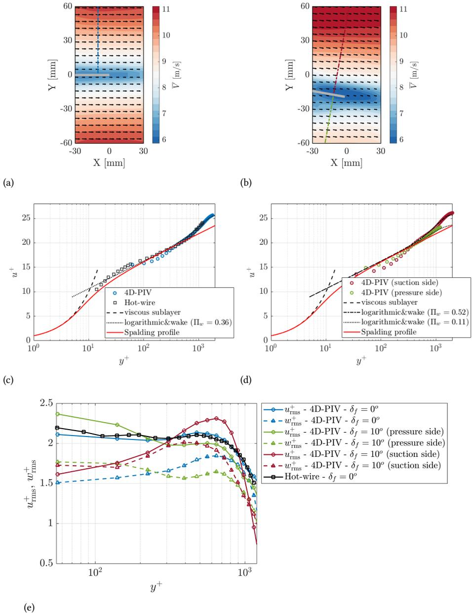
Figure A.2: Mean flow over the trailing edge and boundary-layer mean velocity profile measured at the trailing edge at  $\delta_f = 0^\circ$  (a and c respectively) and  $\delta_f = 10^\circ$  (b and d respectively) and root mean square (RMS) of the stream and spanwise velocity fluctuations (e). The dashed lines in (a) and (b) represent the region of extraction of the boundary-layer velocity profiles.
