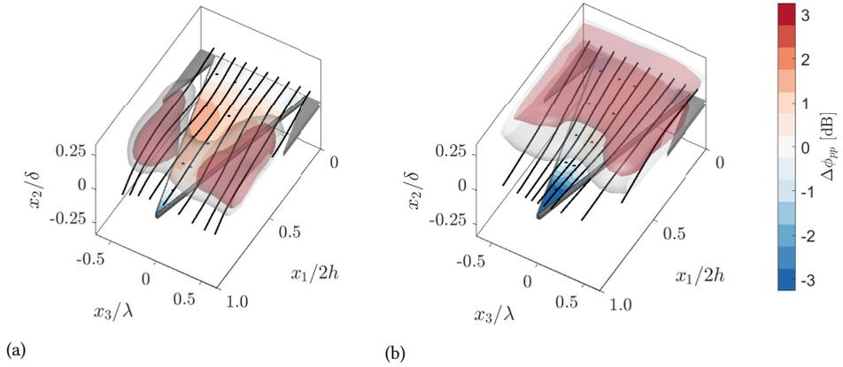
Figure 5.9: Iso-surfaces of the MS-T term (bandpass filtered at  $f/\delta^*/U_\infty = 0.4$ ) compared against the surface pressure measurements from the microphones on the pressure (a) and suction side (b) of the flat plate at  $\delta_f = 10^\circ$ . The iso-surfaces represent non-dimensional levels MS-T of 0.025 (grey surface) and 0.04 (red surface). Pressure fluctuations are taken from Figure 5.4.
