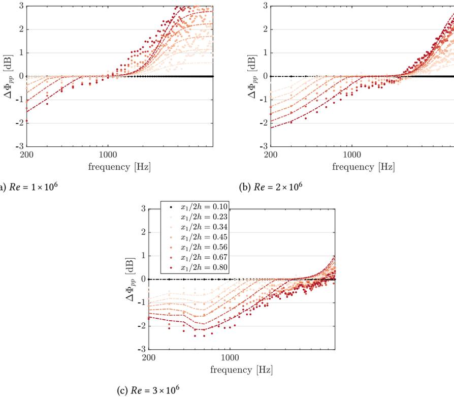
Figure 6.9: Comparison between measured (circular marks) and predicted (dashed-dotted lines)  $\Delta\phi_{pp}$  at sensor positions along the centre of the serration for  $\alpha = 0^\circ$ . Delta values are computed as the difference with respect to the pressure fluctuations measured by the sensor at the centre root of the serration ( $x_1/2h = 0.10, x_3/\lambda = 0.0$ ).
