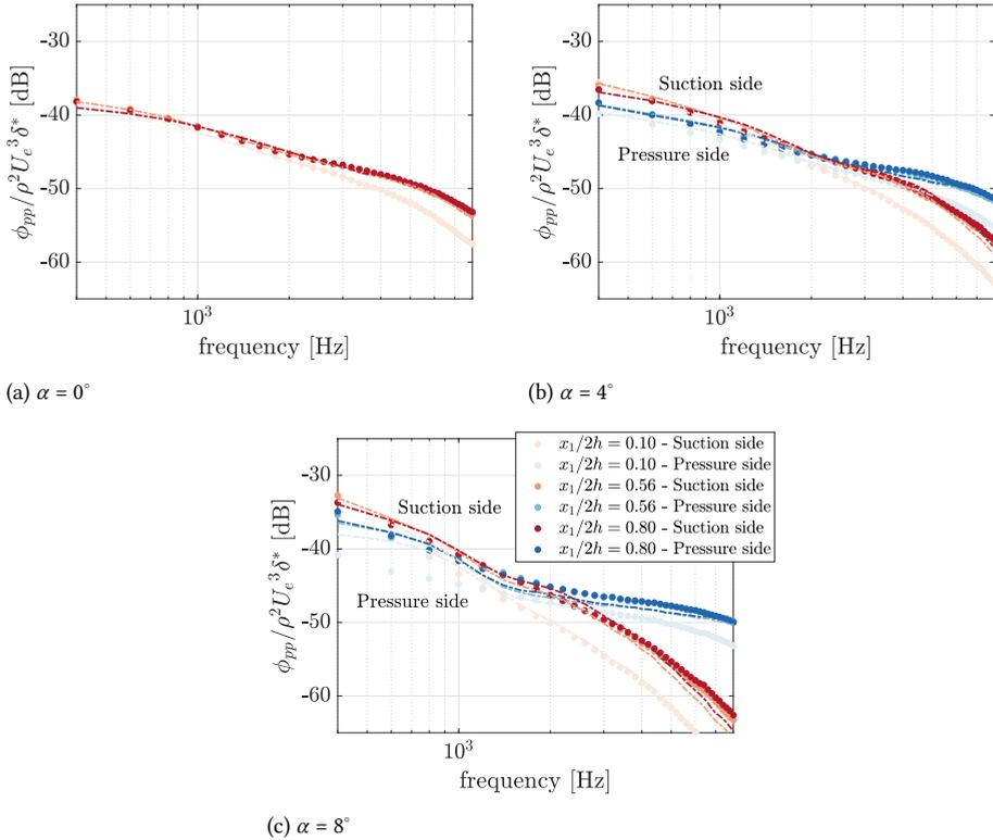
Figure 6.13: Comparison between measured  $\phi_{pp}$  (circular marks) and predicted wall-pressure spectrum (dashed dotted lines) along the serration edge for three different angles of attack ( $Re = 2 \times 10^6$ ). Levels are made non-dimensional with respect to the boundary-layer displacement thickness at  $\alpha = 0^\circ$ . The analytical predictions are created using the spectrum at the centre and root ( $x_1/2h = 0.1$ ,  $x_3/\lambda = 0.0$ ) of the serration as reference.
