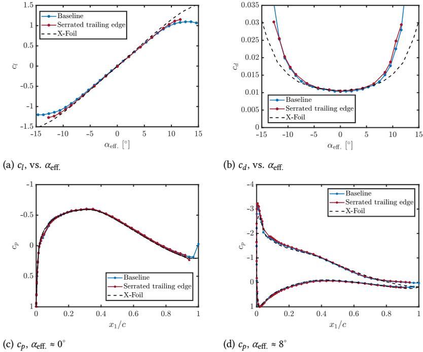
Figure 4.10: Comparison between conditions with and without trailing-edge serrations. (a)  $c_l$ , vs.  $\alpha_{eff}$ , (b) shows the  $c_d$ , vs.  $\alpha_{eff}$ . (c) and (d) shows the pressure distribution along the airfoil surface for angles of  $\alpha_{eff} \approx 0^\circ$ , and  $\alpha_{eff} \approx 8^\circ$  respectively. Measurements are taken at  $Re_c = 3 \times 10^6$ . X-Foil estimations are also provided for reference.
