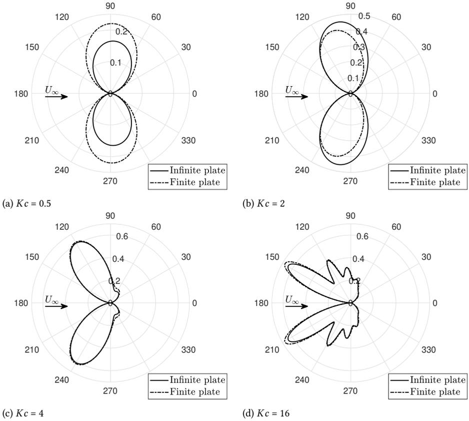
Figure 2.2: Directivity plot for the scattering of an infinite span wing with a straight trailing edge at  $M = 0.2$  at different frequencies. The solid line represents the estimations without back-scattering, and the dashed lines with the back-scattering corrections.
