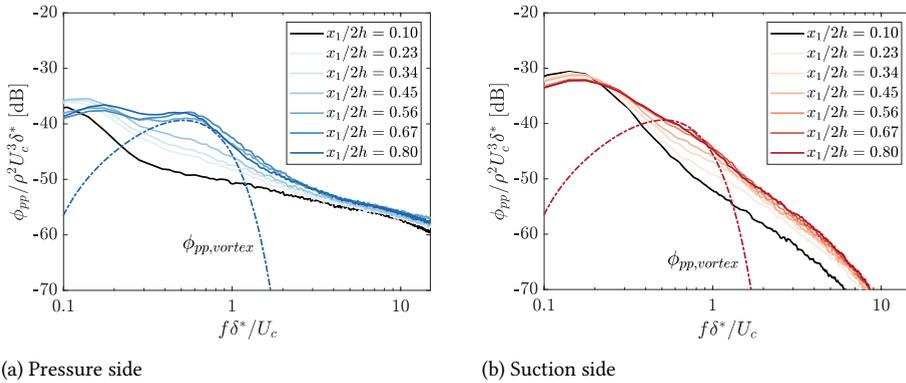
Figure 6.11: Measured variation of the wall-pressure spectrum measured ( $\phi_{pp}$ ) along the serration edge for  $\alpha = 10^\circ$  and  $Re = 2 \times 10^6$ . (a) shows the spectrum along the pressure side and (b) along the suction side. Predicted aerodynamic loading effects are presented in dashed and dotted lines ( $C_v = 5.1 \times 10^{-3}$ ).
