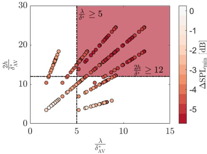
Figure 7.12: Summary scatter plot of maximum noise reduction  $\Delta\text{SPL}_{\min}$  for all sawtooth geometries tested under all angle of attack and flow speed conditions available. The graph also depicts the two criteria for serration design mentioned in this work, i.e.  $2h/\delta^* \geq 12$ , and  $2h/\delta^* \geq 5$
