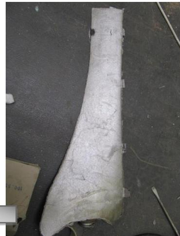
FIGURE 33: RAW SAND-CASTED BLADE
