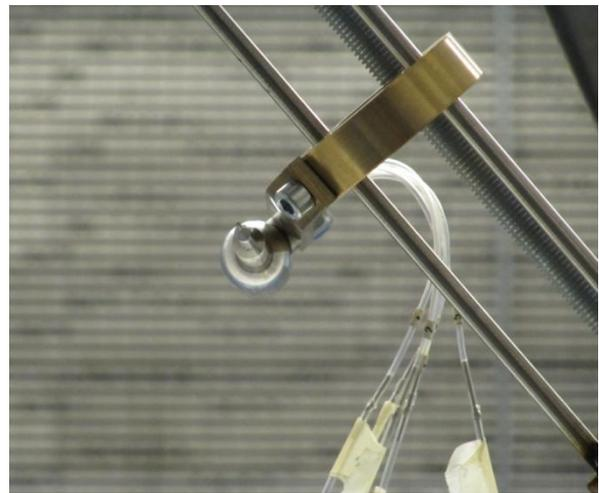
FIGURE 46: 5 HOLE PITOT TUBE
