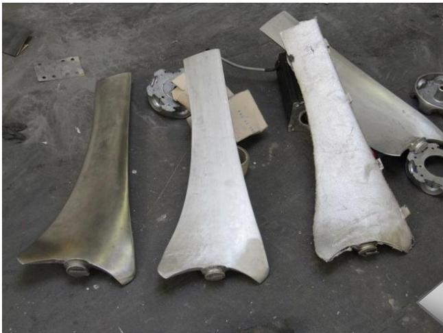
FIGURE 32: VARIOUS STAGES IN GRINDING AND SANDING
