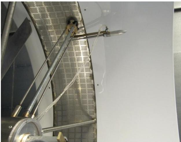
FIGURE 45: TRAVERSING MECHANISM
