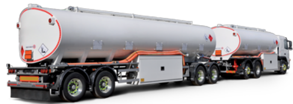
Figure 2.2: Example rigid truck with drawbar trailer (HMK Bilcon, 2016b).
