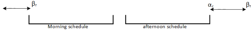
Figure 5.8: Situation where the route departure window lies completely outside of a vehicle schedule, making the route–vehicle combination impossible.
