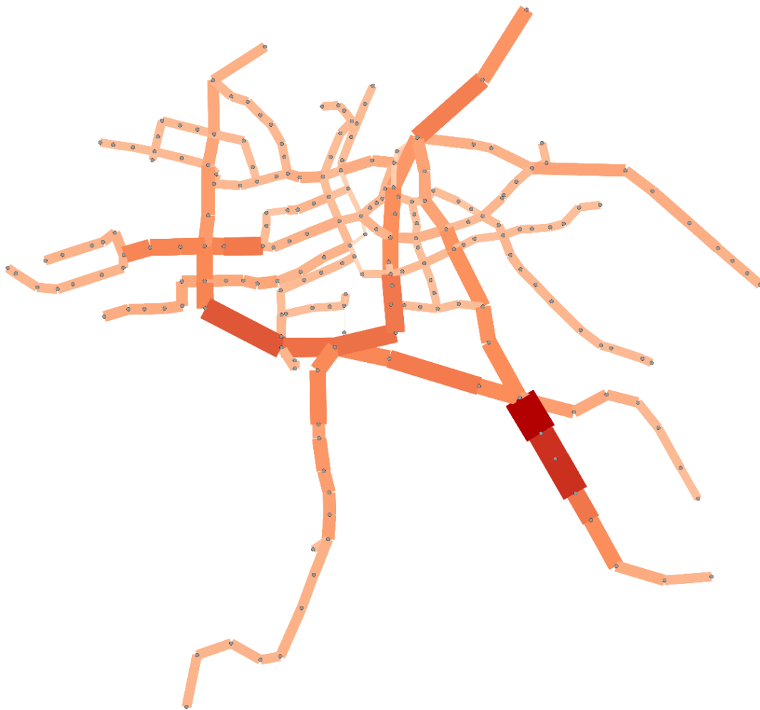
Figure 48 Graph of the Link Criticality indicator (10-100%) for the links in the Amsterdam urban rail bound PT network (Thicker and more saturated red links indicate a higher score)
