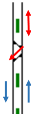
Figure 70 Example of the use of a crossover in case of line cutting
