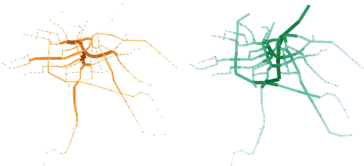
Figure 59 Two attributes representing link centrality: left the L-space link Betweenness centrality, right the L-space link closeness centrality indicator (thicker and more colour saturated links have a higher value)
