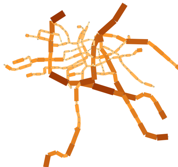
Figure 62 Operational link characteristic as the mean speed on the link (thicker and more colour saturated links have a higher value)
