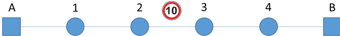
Figure 15 Visualization of a local speed limit on a link in a single line. The blue circles are served stops, the blue squares are terminal stations and the number in the red circle is the local speed limit.
