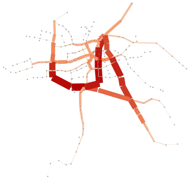
Figure 57 Total bi-directional flow on the links as the passenger demand on the link (thicker and more colour saturated links have a higher value)
