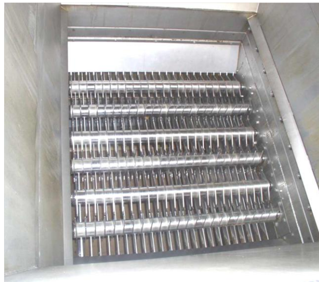
Figure 3.12: Frozen tobacco crusher: clump breaker
