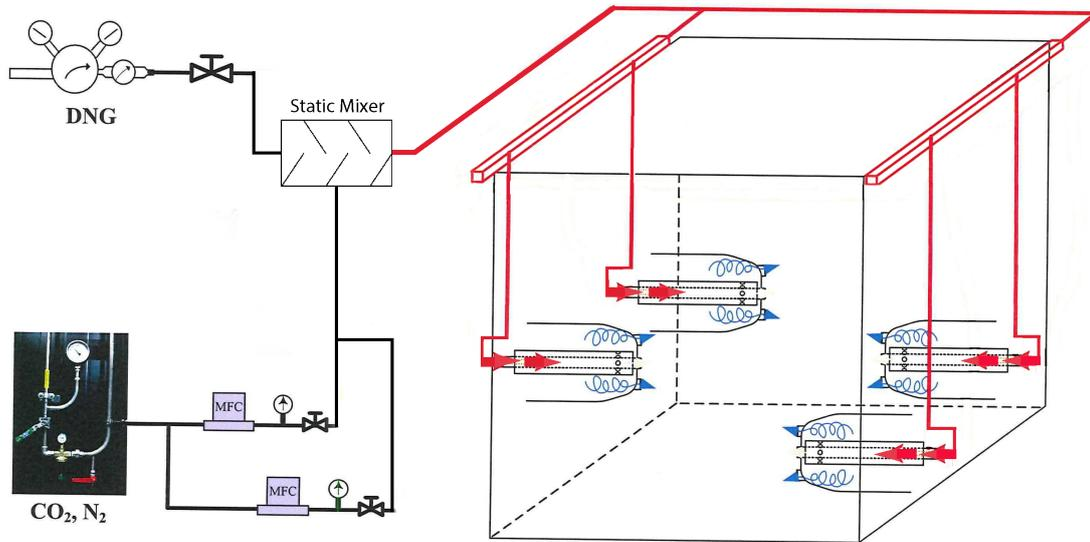
**Figure 3.9:** This figure shows the suggested system where the dilution streams and DNG are premixed in a static mixer and use the current control system during operation.
