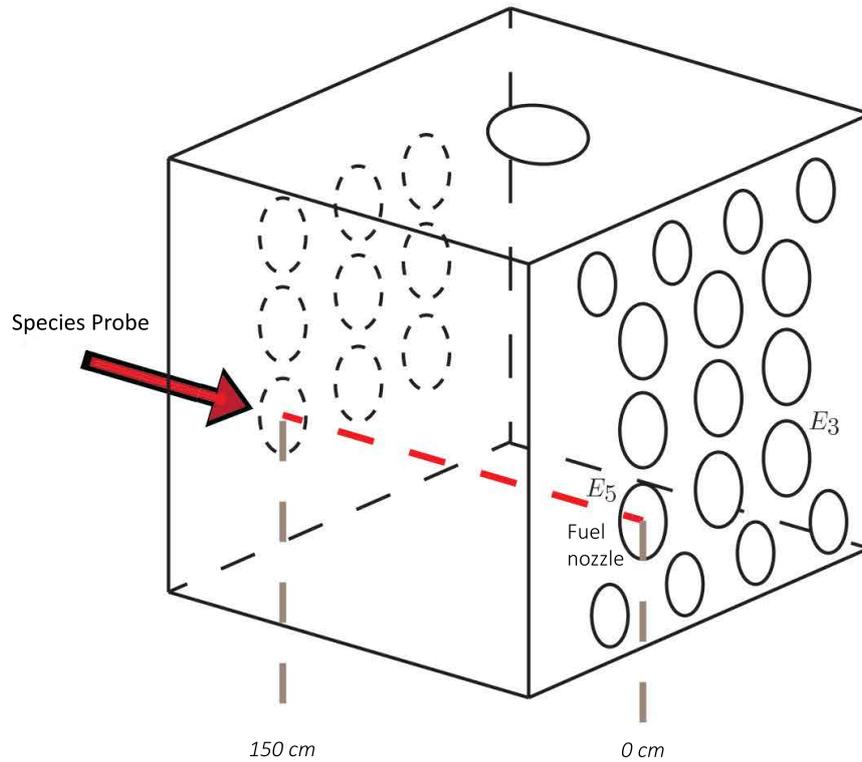
**Figure 3.7:** Shown here in red is the line along which the species probe is inserted into the furnace from the 150cm mark up until 5cm away from the fuel nozzle.
