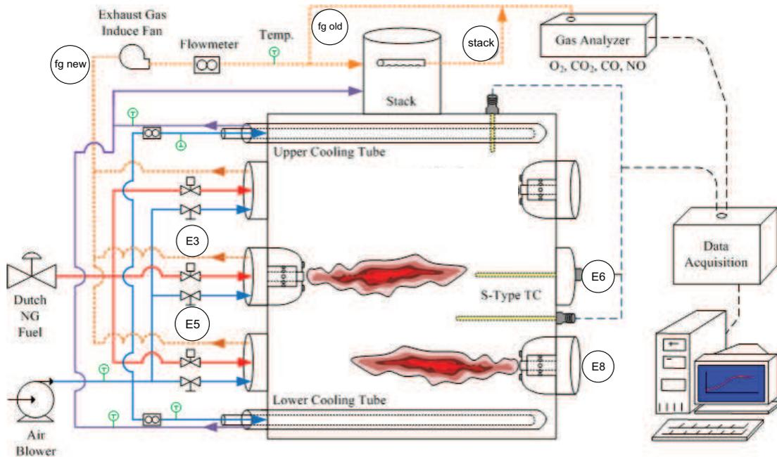
**Figure 3.3:** Overview of the furnace, where the measuring points have been indicated as circles. The species probe point has been omitted for the sake of clarity of the picture. Image adjusted, original made by E.S. Cho.
