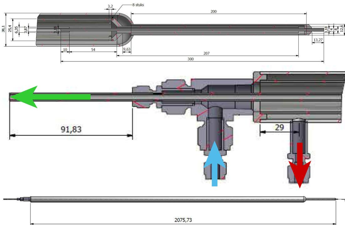
**Figure 3.6:** Technical drawings of the species probe with a magnified view of the top (top) and end (middle) sections and a global view (bottom). All dimensions in mm. Flows of flue gas (green) and water in & out (blue, red) are shown in the middle picture.
