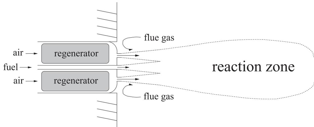
**Figure C.1:** In this figure the entrainment of flue gases can be seen which form the near burner zone when combustion initiates and subsequently flows over into the reaction zone. Picture made by B. Danon.
