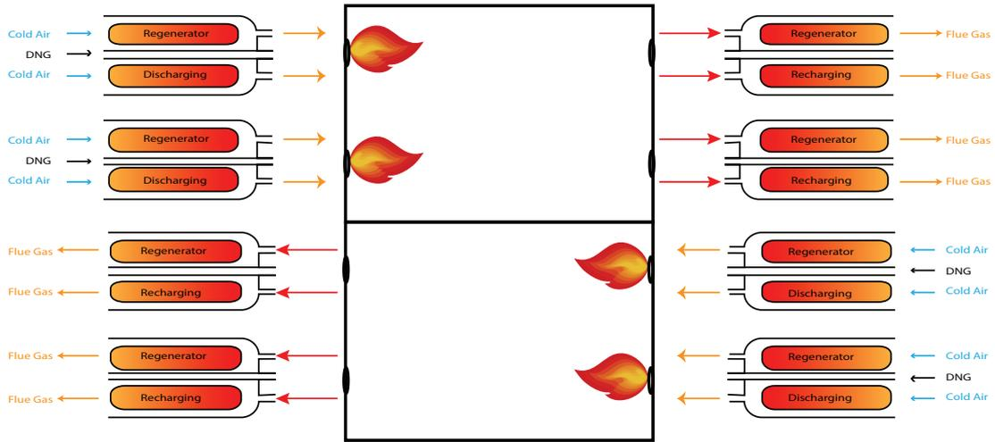
**Figure 1.1:** Alternating operating mode of the MEEC regenerative combustion furnace with temperature gradients displayed over the ceramic honeycomb heat exchangers.
