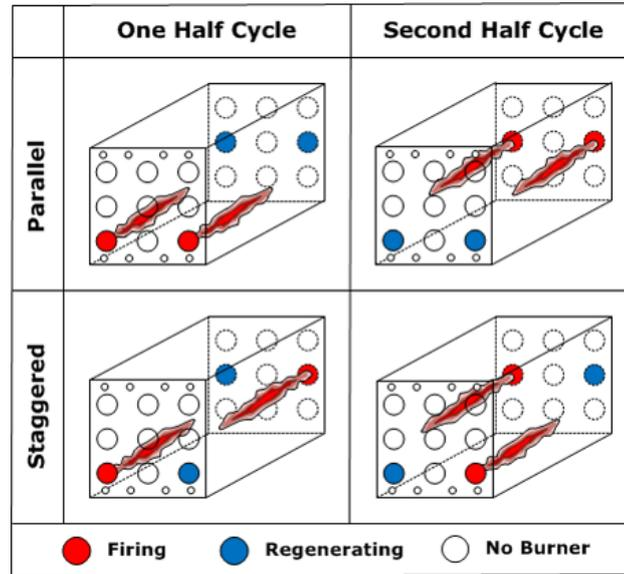
**Figure 4.1:** Overview of the firing modes used. The parallel mode is shown on top for both parts of the cycle and the staggered 1 mode is shown on the bottom.
