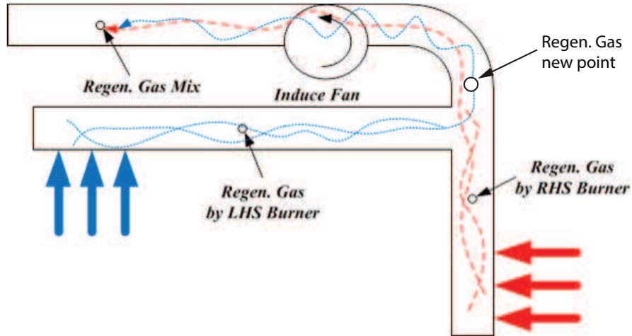
**Figure 3.4:** This figure shows the situation for the flue gas streams around the inducer fan as well as the new measurement location. Figure adapted from E.S. Cho.
