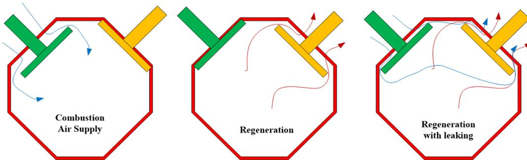
**Figure 3.10:** This figure shows the pathways of the air through which it can escape (*leakage*) during several steps of the burner cycle. Figure made by E.S. Cho.
