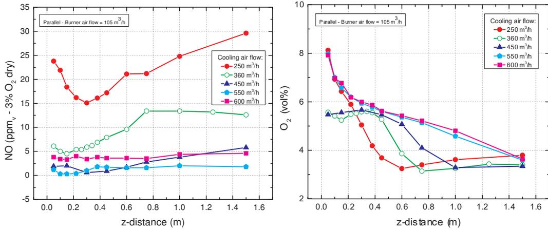
**Figure 6.2:** Parallel firing mode. On the left the NO concentration is shown as a function of species probe insertion depth for several cooling air flow rates with constant burner air flow rate. The oxygen concentration can be seen on the right for the same cases. Burner is located at  $z = 0$
