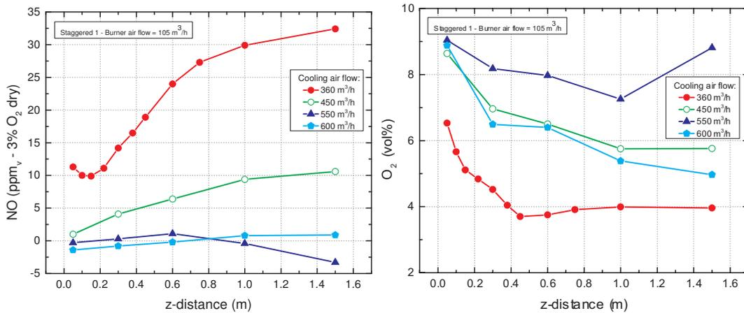
**Figure 6.6:** Staggered 1 firing mode. NO and oxygen concentration are shown on the left and right in this figure. Both are displayed as a function of the insertion depth of the species probe for several cases of cooling air flow rate.
