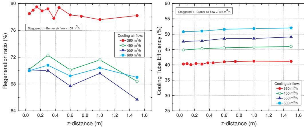
**Figure 6.8:** Staggered 1 firing mode. The regeneration rates (left) and cooling tube efficiencies (right) as a function of species probe insertion depth for varying cooling air flow rates are shown in this figure.
