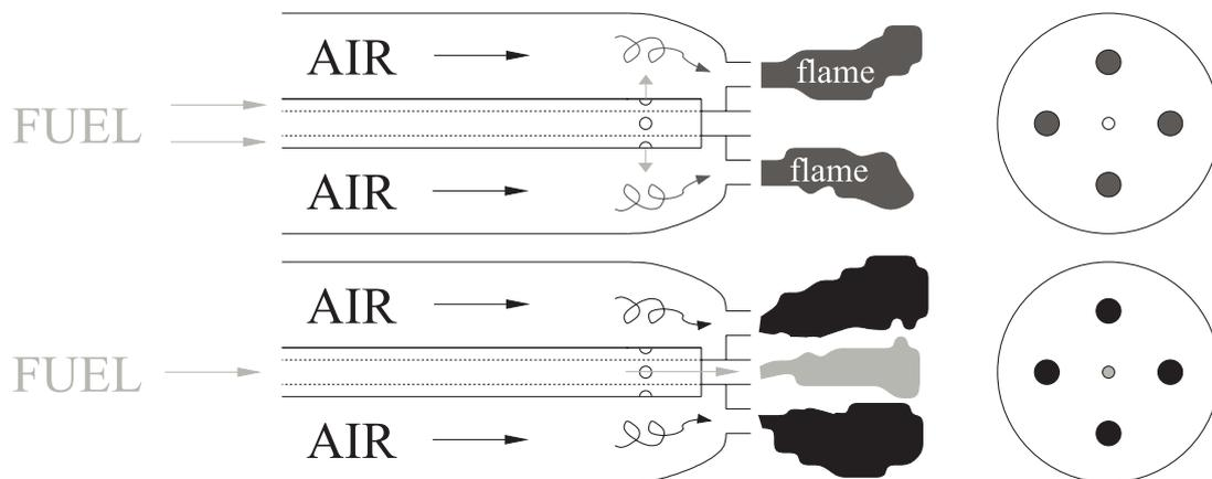
**Figure B.1:** In this figure the difference is shown between the flame (top) and the FLOX (bottom) firing modes. Picture made by B. Danon.
