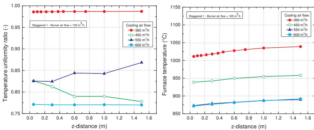
**Figure 6.5:** Staggered 1 firing mode. This figure shows the temperature uniformity (left) and furnace temperature (right) as a function of species probe insertion depth for varying cooling air flow rates.
