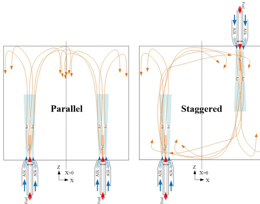
**Figure 4.2:** Theoretical 2D flow patterns in the furnace during the parallel and staggered firing modes. Figure made by E.S. Cho.
