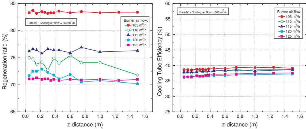
**Figure 6.12:** Parallel firing mode. The regeneration ratio expressed as percentage as a function of species probe insertion is displayed in the left graph for several burner air flow rates. The cooling tube efficiency is shown on the right for the same cases.
