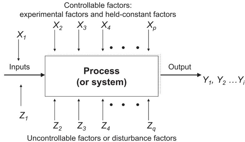
**Figure 2.3:** In this figure a representation is given for a process under experimentation. Factors that affect the system are divided into controllable (Xs) and uncontrollable (Zs) and result in the responses (Ys) of the system [13].
