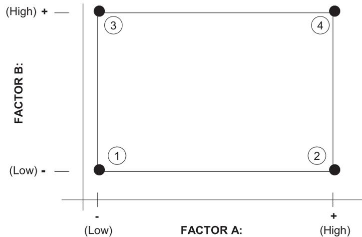
**Figure 2.2:** An example of the classical type of factorial design is displayed in this figure. The main drawback of these designs are the increasing complexity and required runs for a high number of factors and responses.
