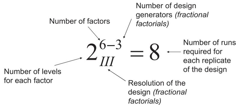
**Figure 2.1:** An example of a two-level (1/8 fractional) factorial design [13].
