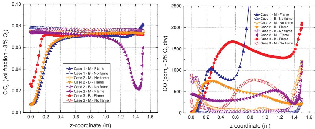
**Figure 6.15:** The  $CO_2$  concentration can be seen on the left for the three cases as described in Table 5.1. The right graph shows the CO concentration along the z-axis. This axis is the same as used for the experimental campaign so only the position of the flame changes depending on the presented curve.
