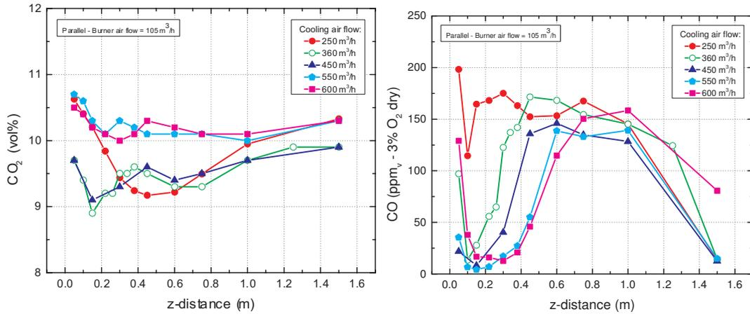
**Figure 6.3:** Parallel firing mode. In the left graph the species concentration for  $CO_2$  is displayed as a function of species probe insertion depth for several selected cooling air flow rates. On the right the CO concentration is shown for the same cases. Burner is located at  $z = 0$
