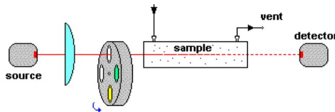
**Figure 3.5:** Basic representation of the working principle of the NDIR detection method [8].
