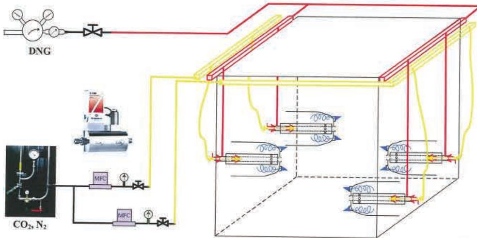
**Figure 3.8:** Current state of furnace. The red lines show the DNG supply while the yellow lines show the  $CO_2$  or  $N_2$  supply. Figure made by E.S. Cho.
