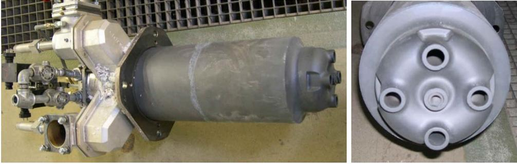
**Figure 3.2:** Different views of the REGEMAT CD 200 type regenerative burners, manufactured by Wärmeprozessstechnik GmbH.
