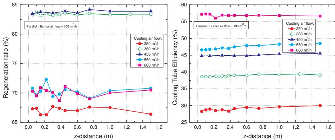
**Figure 6.4:** Parallel firing mode. The regeneration rates (left) and cooling tube efficiencies (right) as a function of species probe insertion depth for varying cooling air flow rates are shown in this figure.
