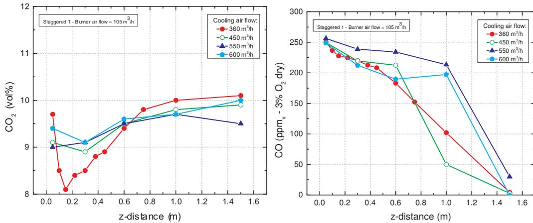
**Figure 6.7:** Staggered 1 firing mode. In the left graph the species concentration for  $CO_2$  is displayed as a function of species probe insertion depth for several selected cooling air flow rates. On the right the CO concentration is shown for the same cases.
