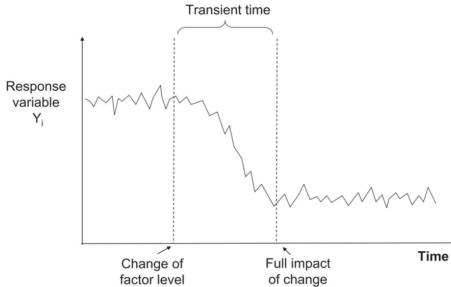
**Figure 3.11:** This is an illustration of the transient time required during continuous processes such as in the MEEC furnace before an induced change to the system is stabilized in the response [13].
