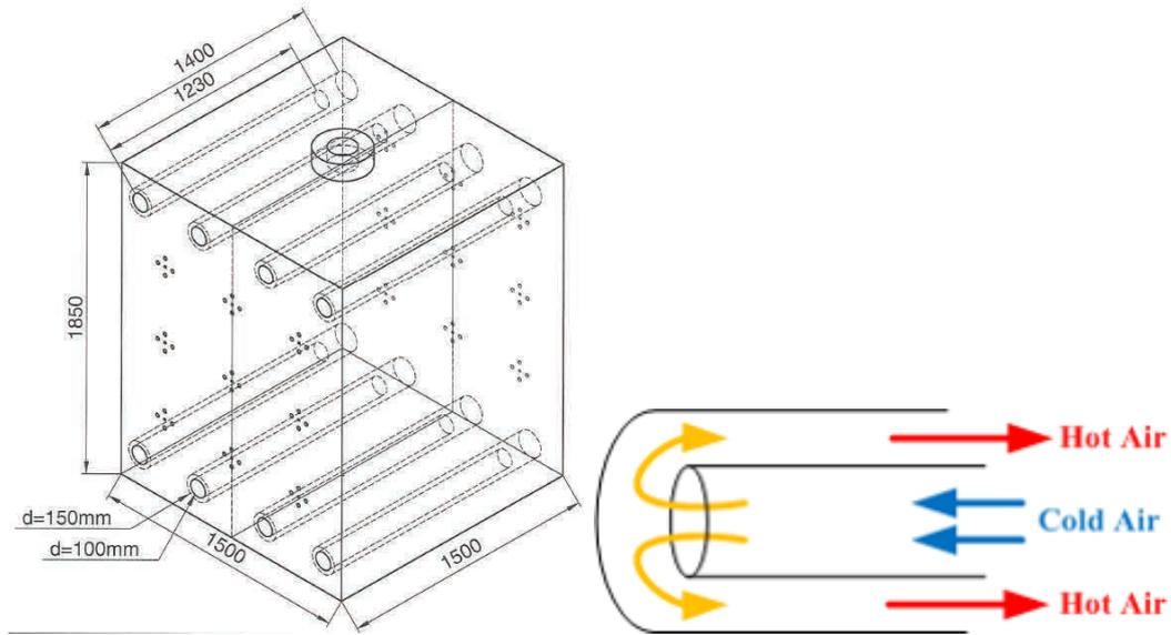
**Figure 3.1:** On the left a sketch of the MEEC furnace. All dimensions are in mm. On the right the air flows in the cooling tubes are shown schematically.
