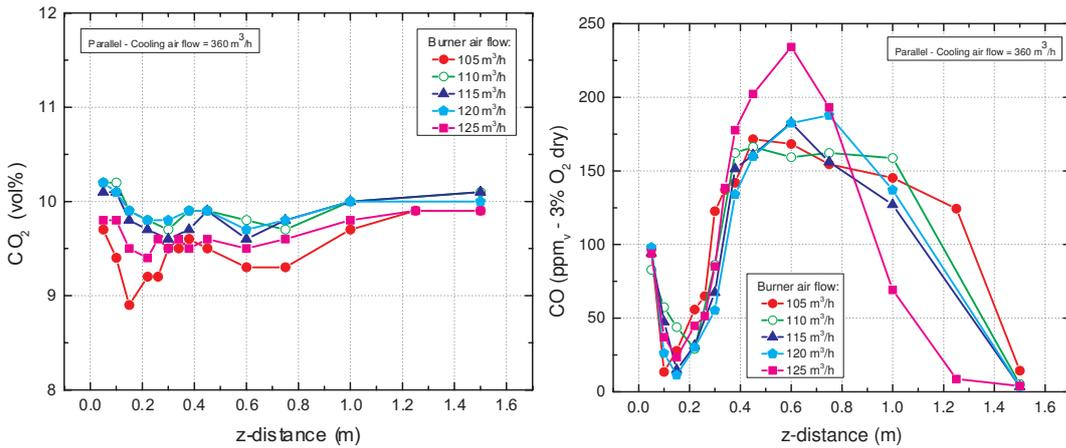
**Figure 6.11:** Parallel firing mode. The CO<sub>2</sub> species concentration profiles for the species probe insertion are displayed on the left for several burner air flow rates. The CO profiles are displayed on the right hand side of the figure for the same cases.
