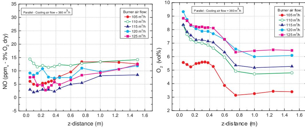
**Figure 6.10:** Parallel firing mode. On the left the NO species concentration is shown as a function of species probe insertion depth for several burner air flow rates. The oxygen concentration for the same cases is displayed on the right.
