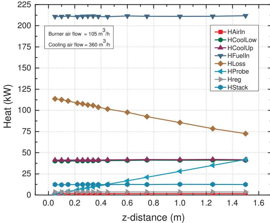
**Figure D.1:** This figure shows the heat input and outputs for the parallel firing mode with  $360 \text{ m}^3/\text{h}$  cooling air rate and  $105 \text{ m}^3/\text{h}$  burner air flow rate. The effect of the linear cooling capacity of the probe is clearly visible on both the HProbe and HLoss lines.
