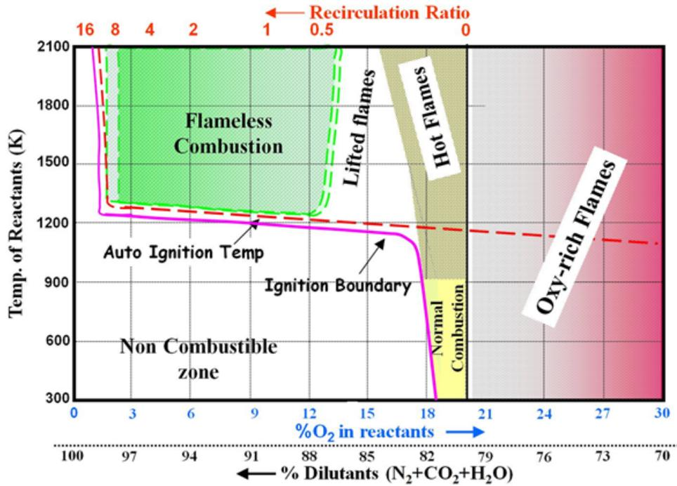
**Figure 1.2:** Diagram showing the operating regimes for flameless combustion [8].
