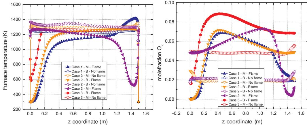
**Figure 6.14:** The furnace temperature is seen on the left for the three cases as described in Table 5.1. The right graph shows the oxygen mole fraction along the z-axis.
