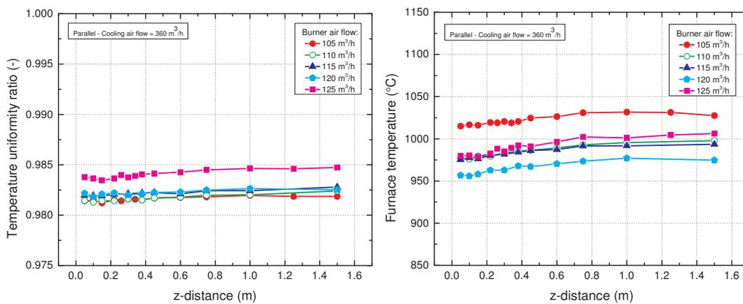
**Figure 6.9:** Parallel firing mode. In the left graph the temperature uniformity is shown as a function of the species probe insertion depth for several burner air flow rates. The furnace temperature is displayed on the right side for the same set of parameters.
