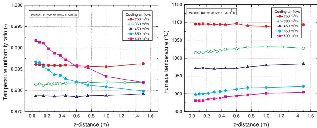
**Figure 6.1:** Parallel firing mode. The temperature uniformity (left) and furnace temperature (right) for several cooling air flow rates and constant burner air flow rate are shown as a function of species probe insertion depth. Burner is located at  $z = 0$ .
