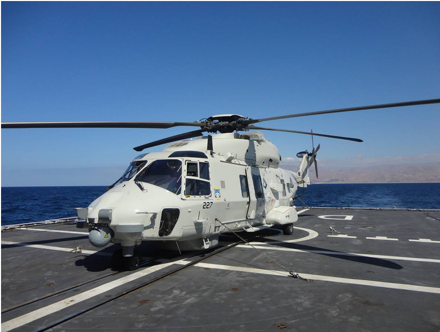
Figure 2-26; Helicopter secured and lashed on deck
