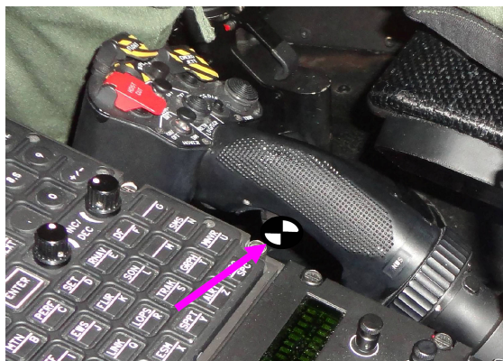
Figure E-4; Example control reference point - collective
