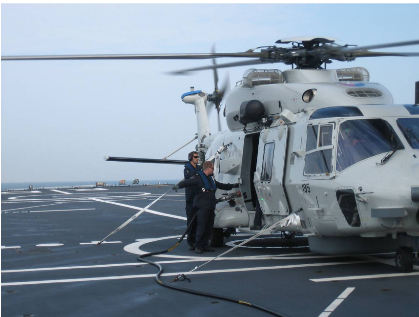
Figure 2-27; Helicopter conducting Rotors Running Refuelling (RRR)
