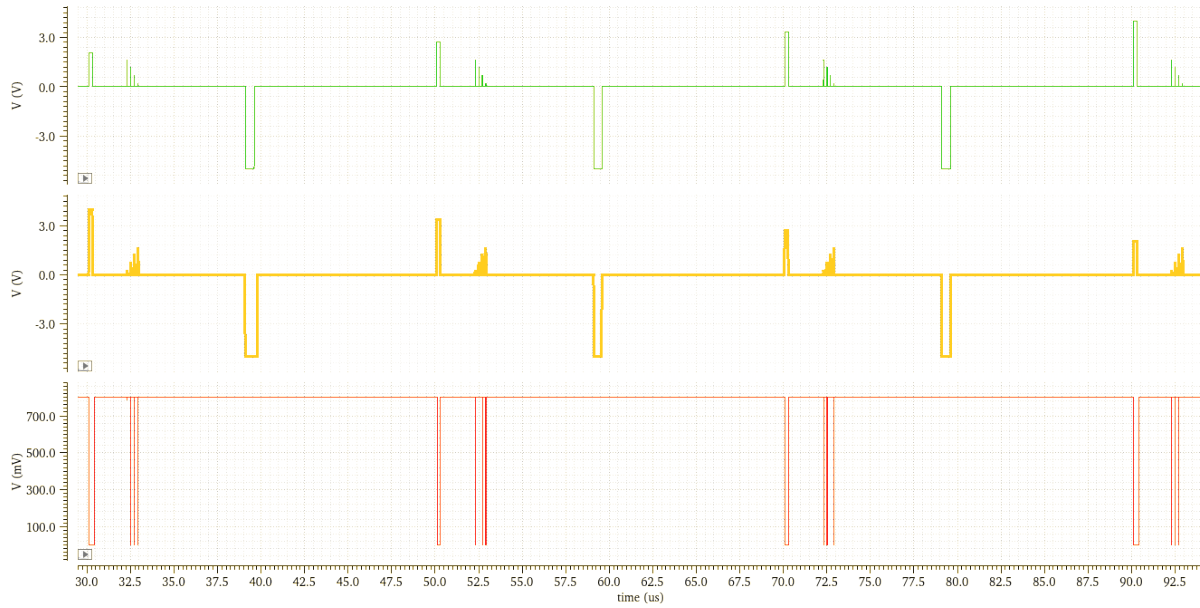
Figure 6.5: Pulse plot during simulation. The first two plots are the write/read pulses, while the last one is the output from the SA. The negative pulses are erase operations, followed by a relatively high positive pulse which programs the cell. The subsequent short pulses are the read operations. Notice the differential signals between the input terminals.
