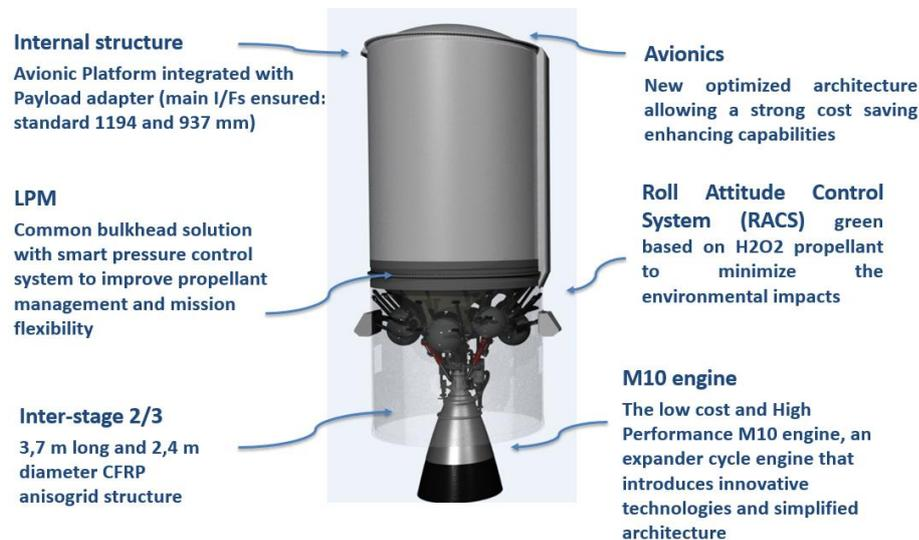
Figure 5.2: M10 engine characteristics given by [29]
