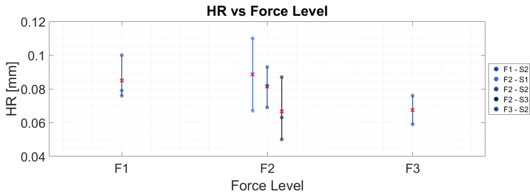
Figure 5.48: h_R for different force levels, including speed level subsets
