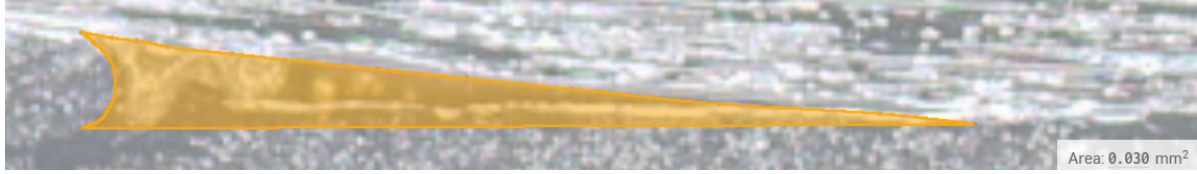
Figure C.4: Traced area for gap three, left void
