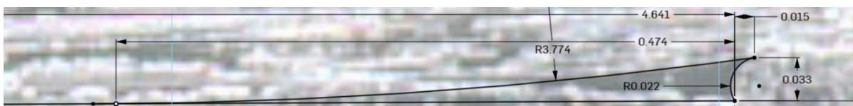
Figure 5.25: Parametrisation of gap three, right void
