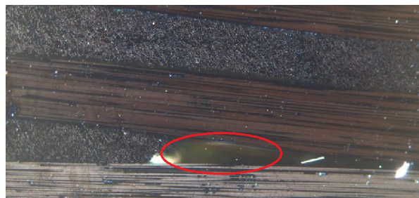
Figure 2.23: Manufactured sample with highlighted void: bottom left of figure 2.20
