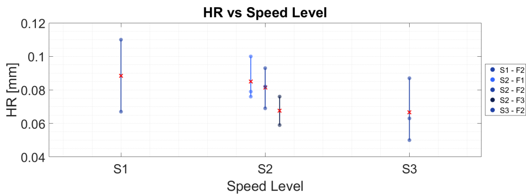
Figure 5.49: h_R for different speed levels, including force level subsets
