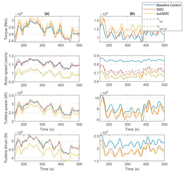
Fig. 6. SMC ( $\lambda_{opt} = 7.55$ ) and subSMC ( $\lambda_{sub-opt} = 6.795$ ) using the UKF-based EWS compared to the baseline controller at mean inflow wind speed of 9 m/s: (a) the upstream and (b) the downstream NREL 5MW RWT
