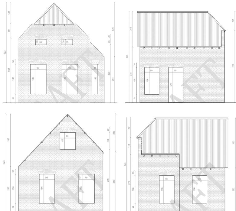
Figure 4.17: Elevation views of the house from four lateral sides (in *cm*) (Graziotti et al. [2016])
