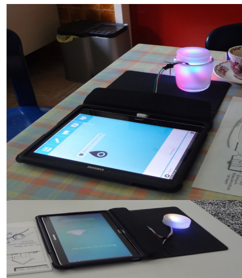
Figure 4-24 Showing possibilities for the reminder signal and progression indication with colored light interaction.
