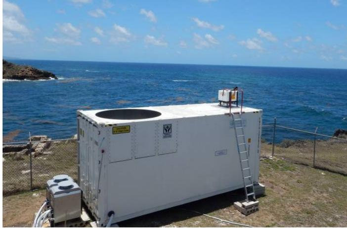
Figure 5: This figure shows the CORAL Ka-Band Cloud Radar at the Barbados Cloud Observatory. We use its measurements for the purposes of this thesis. From ref. [7].
