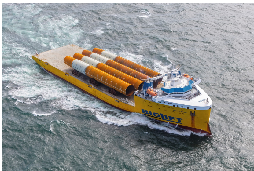
Figure 1.1: Example of large monopiles being carried by MC-class
