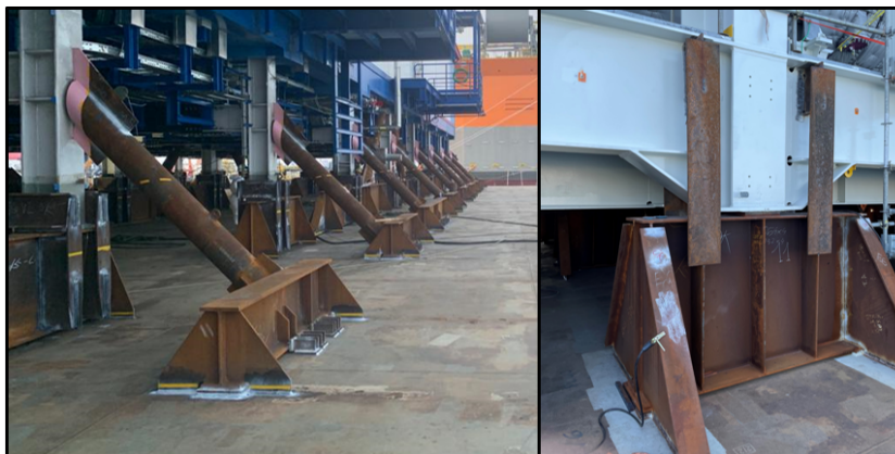
Figure 2.3: Usage of shear plates and push-pull bars in the sea-fastening system on the MC-class vessels
