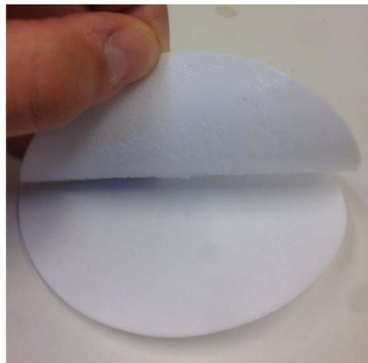
Picture 4.7 Two layers of Teflon sheets stick to each other after grease application
