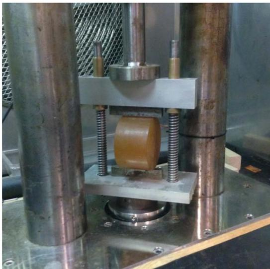
Picture 4.3 Testing head with loading strips and calibration silicon specimen
