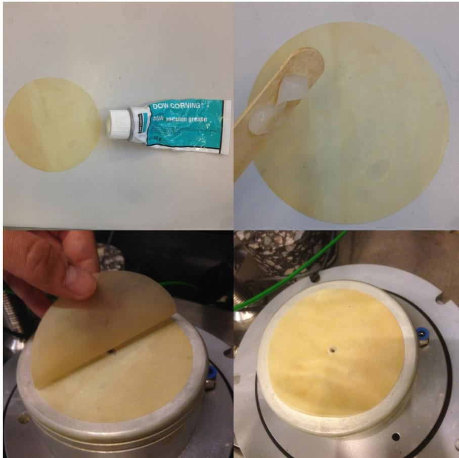
Picture 4.9 Latex membrane and high vacuum grease (top left), spreading 1 gram of grease (top right), grease in between the two latex layers (bottom left), bottom plate (bottom right)
