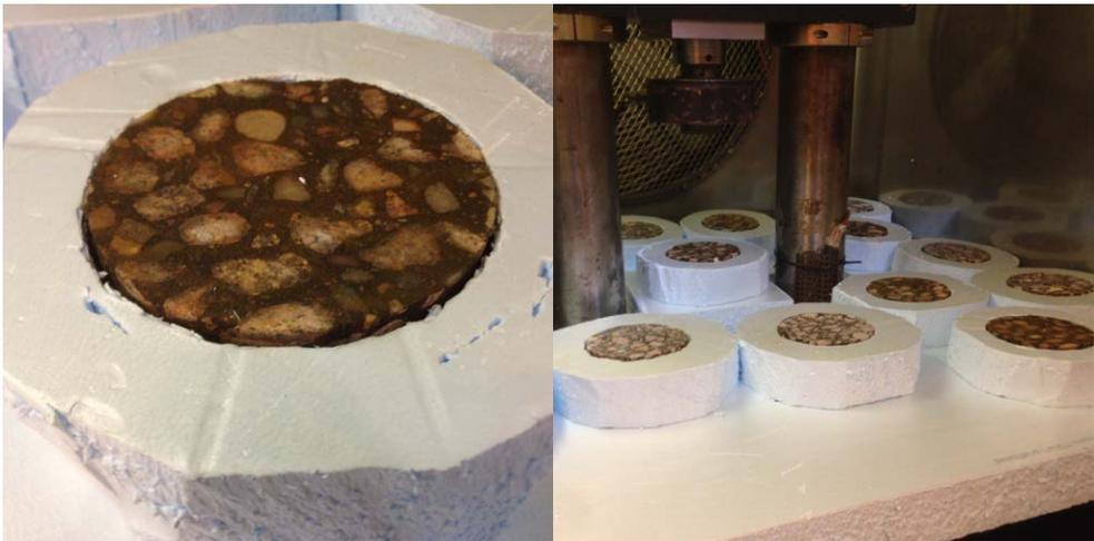
Figure 4.6 Insulation mould (left), and thermal loading chamber (right)
