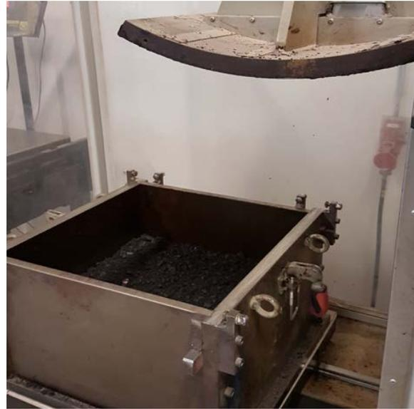
Picture 4.2 Compression device used for the slabs' compaction
