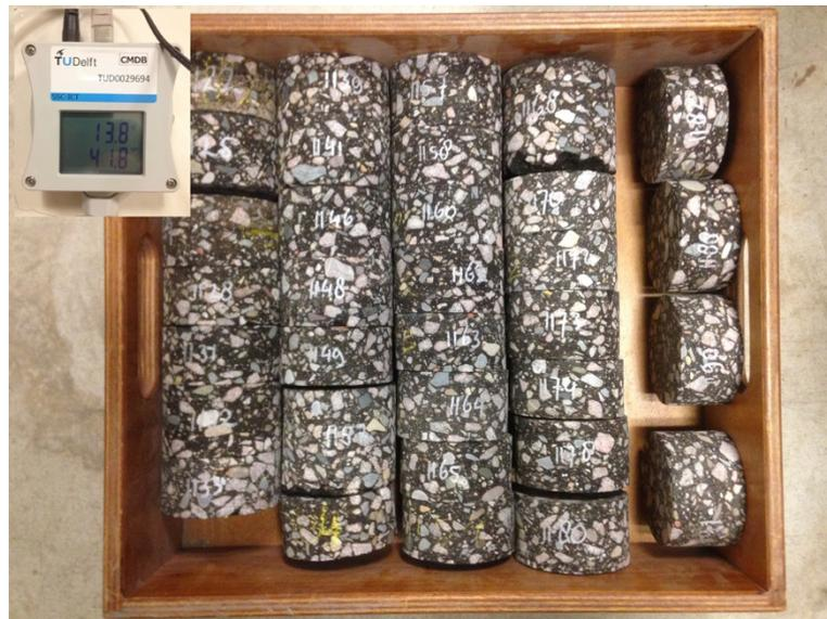
Picture 4.1 Specimens storing conditions at TU Delft
