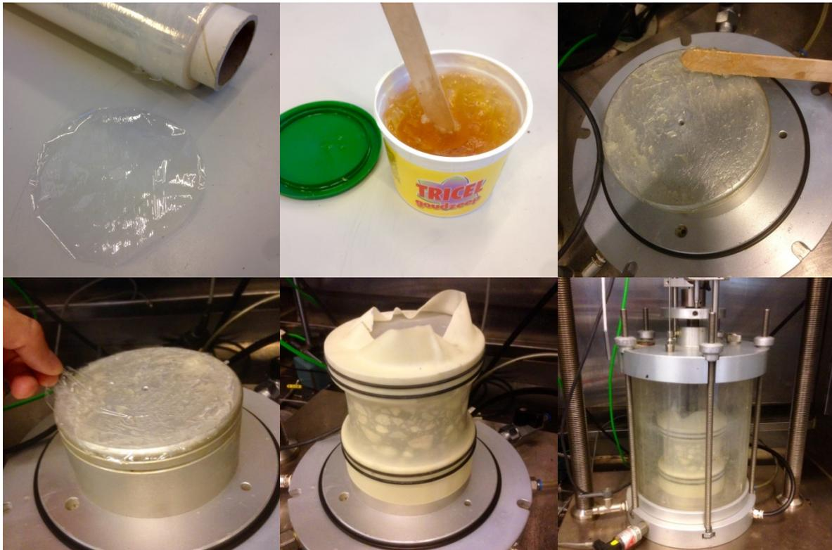
Picture 4.6 Wrapping plastic (top left), conventional soap (top middle), spreading of soap on the bottom plate (top right), placement of plastic on the soap (bottom left), specimen mounted with latex membrane (bottom middle), equipment ready for testing (bottom right)
