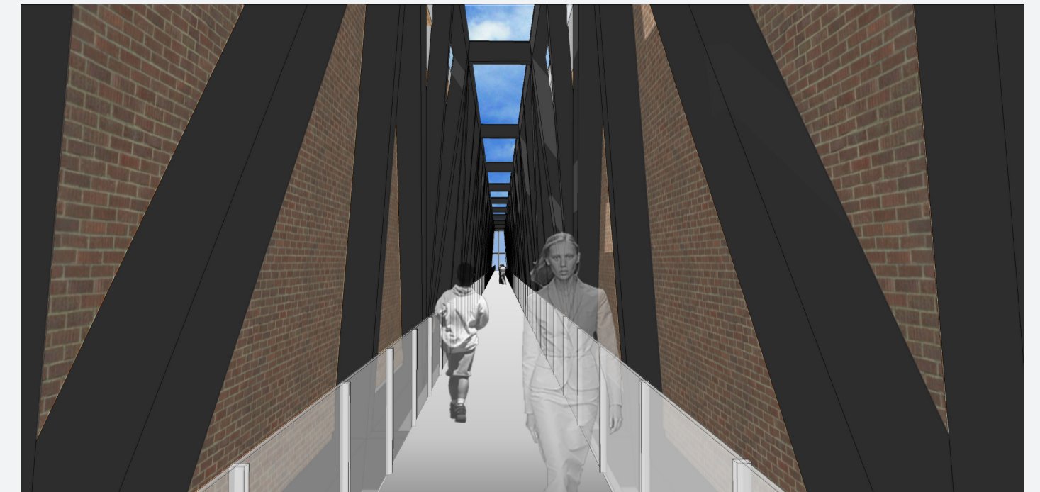
Corridor within the truss beam frame (3rd floor)
