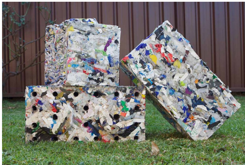
Figure 4.6: Recycled HDPE compressed into blocks (source: ByFusion)
