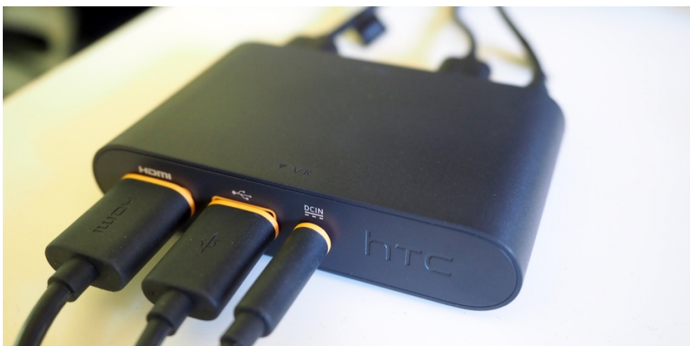
Fig. 8: HTC Vive Link Box, the interface between the PC and the HTC Vive. Available through: https://c.slashgear.com/wp-content/uploads/2016/04/htc-vive-review-4.jpg
