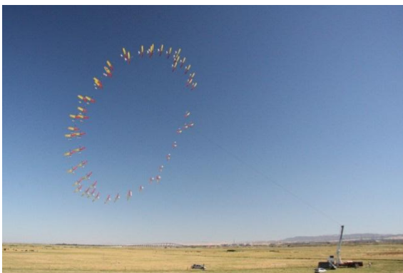
FIGURE 2-4, DRAG POWER CONCEPT OF MAKANI POWER [15]
