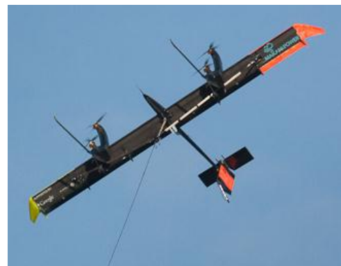
FIGURE 2-5, DRAG POWER CONCEPT, GENERATORS MOUNTED ON WING [15]
