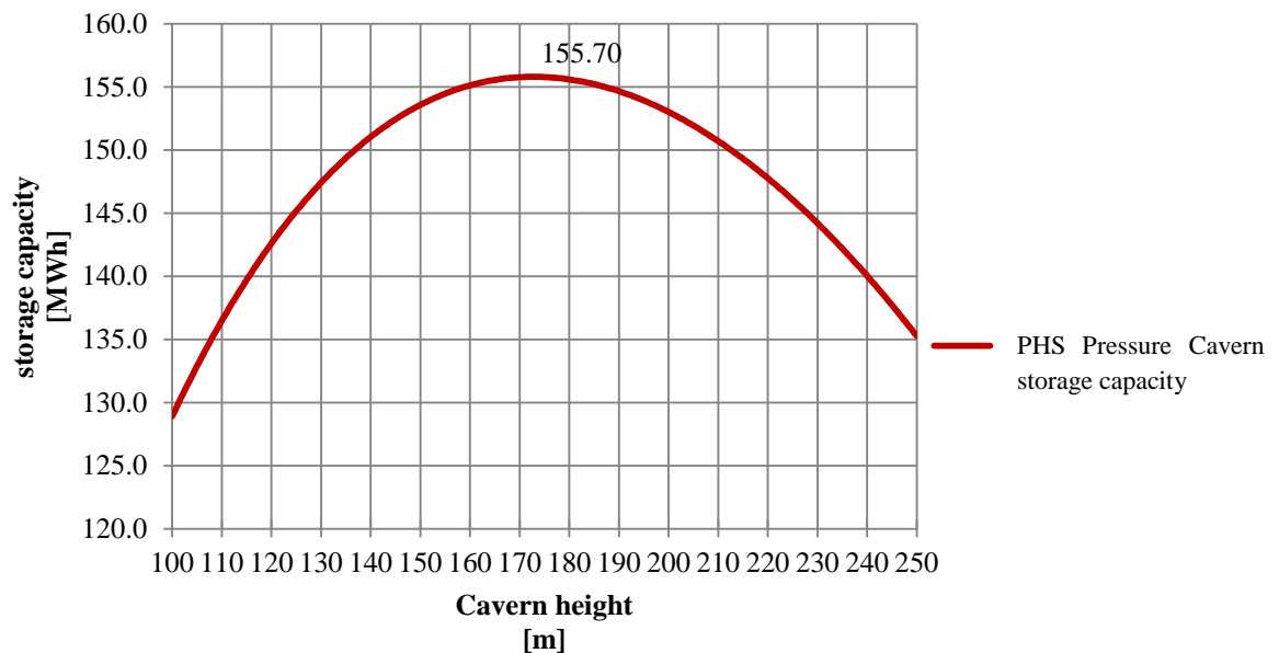
FIGURE 62 - CHANGE OF ENERGY STORAGE CAPACITY FOR DIFFERENT CAVERN HEIGHTS
