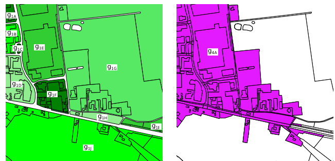
(a) Attractiveness regions are formed by removing the road objects and uniting all connected components. (b) The objects (in purple) belong to an urban region (obtained from an external source).
