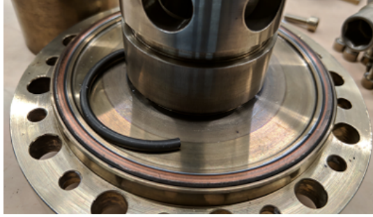
Figure 3.12: A damaged O-ring close to the venting holes in the FOV, possibly cut when pinched by the sliding cylinder when the valve was closed.
