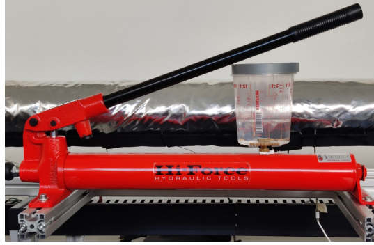
Figure 5.10: Manual pump used for charging the CT; the measuring jar is connected to the pump through the inlet port.
