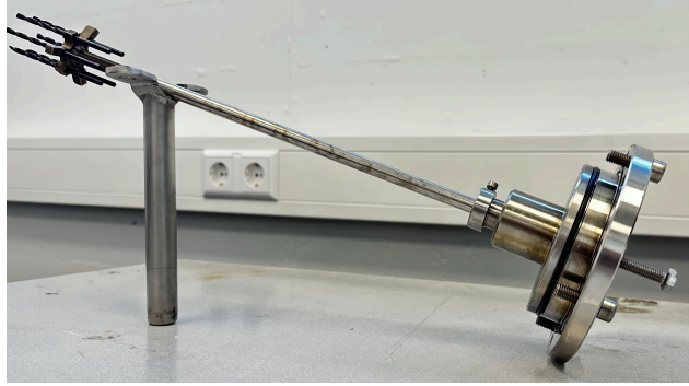
Figure 5.5: Photograph of the breaking pin assembly attached to the LPT end plate.
