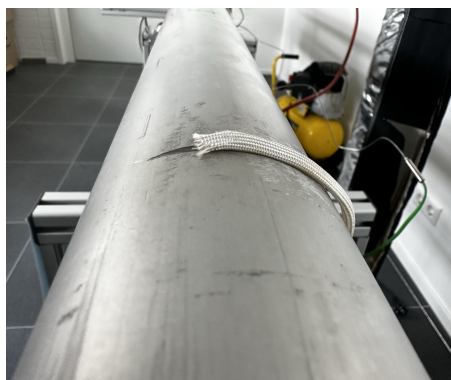
Figure 5.7: Thermocouple attached to the aluminum shell in the ASTER. The thermocouples are placed within a heat resistant fabric sheath to prevent any damage to the heating blankets.
