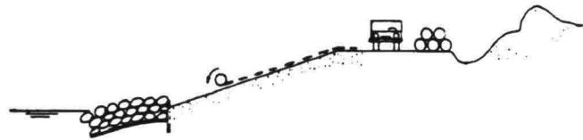
Figure 13.18 Rolling out geotextile
