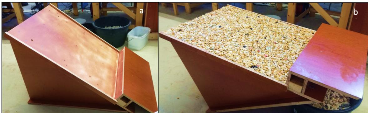
Figure 4.4: Slope preparation a) Wooden slope b) After gluing the stone layer
