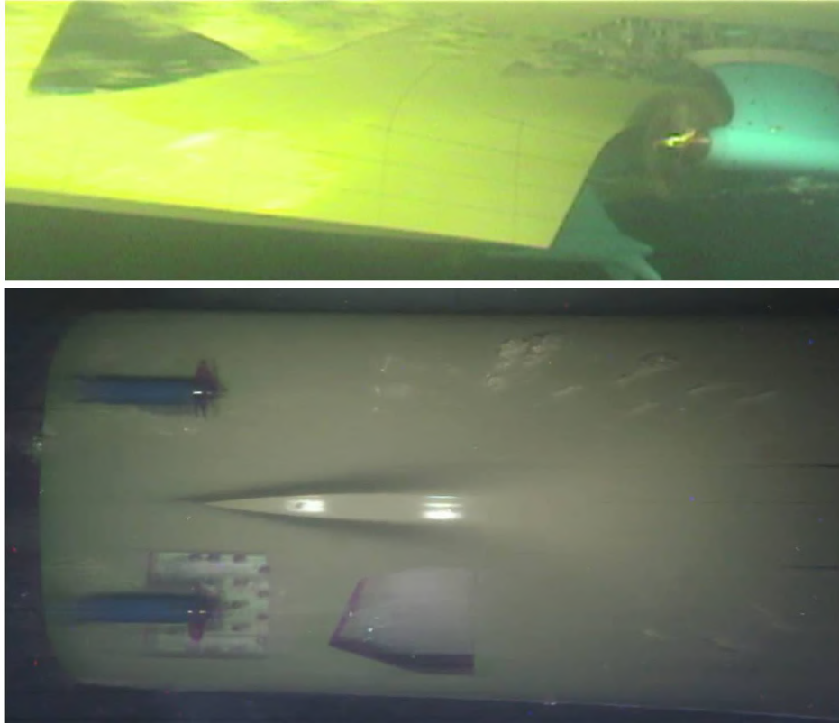
Figure 6.2: Cruise ship: propeller observations with air on at 14 knots during model tests.
