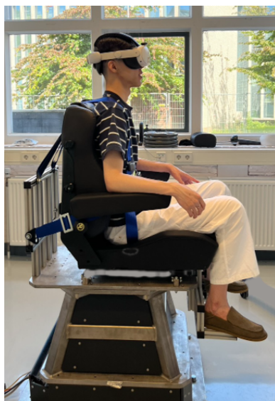
(a) A secured participant at the starting position of the Keshner test. His ears were adjusted close to the rotational axis of the seat to the experimenter's best. The HMD with IMU attached had already been equipped. The participant was asked to face ahead with reference of his proprioception. The headset was removed to avoid the HMD. The back, arms, and feet lay on the backrest, armrest, and footrest, respectively; thereby, the entire trunk was supported by the seat at most.
