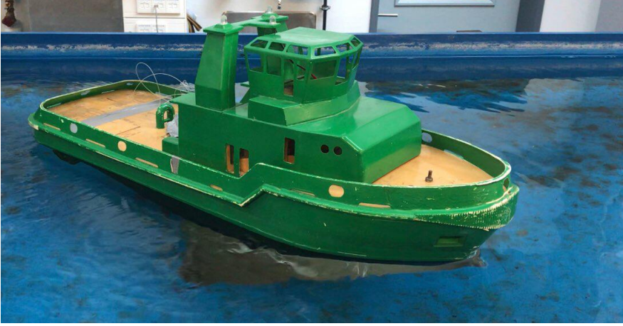
Figure 5.2: Tito-Neri: a harbor tug 1:30 replica model [121].
