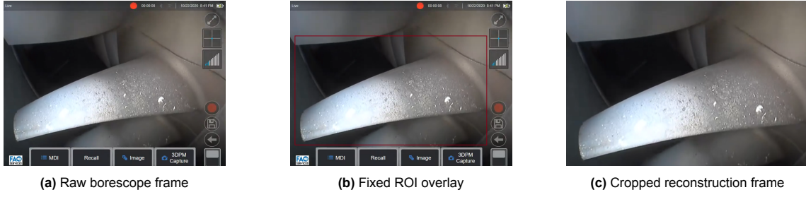
Figure 3.3: Preprocessing and fixed ROI cropping. The raw borescope frame contains endoscope interface elements and peripheral image regions that do not belong to the turbine surface. The fixed ROI removes these non-structural regions and produces the cropped frame used for the later reconstruction stages.
