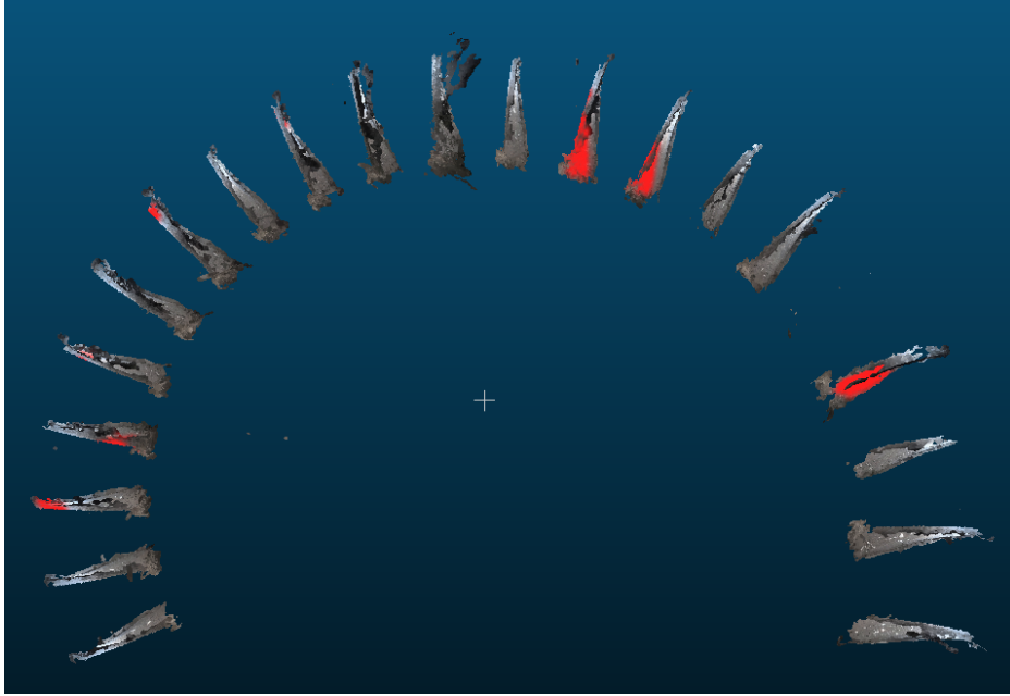
Figure 3.7: Example of the final 3D inspection representation used for comparison. Defect evidence is displayed directly on the reconstructed blade surfaces as colored regions, which provides a geometry-aware inspection view.
