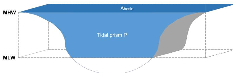
**Figure 2.2:** Schematisation of the tidal prism, which is the water volume between Mean Low Water (MLW) and Mean High Water (MHW) that flows in and out of the tidal inlet during each tidal cycle.
