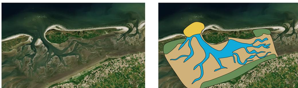
**Figure 2.1:** System components of a tidal inlet, where the ebb-tidal delta is displayed in yellow, the channels in blue, the tidal flats in brown and the salt marshes in green.
