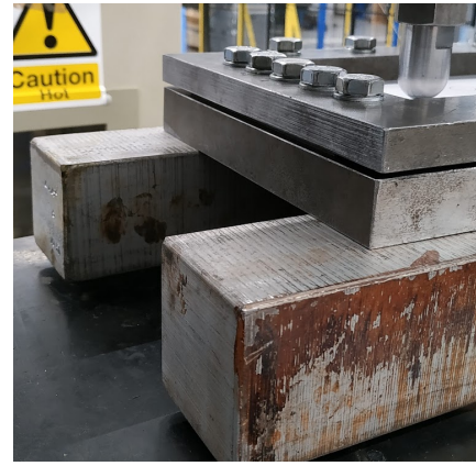
Figure 3.5: Metal blocks supporting the clamp
