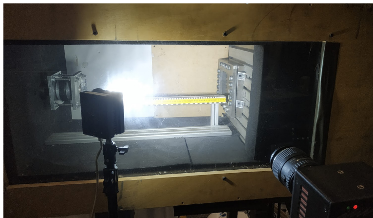
Figure 3.6: Ice impact set-up with high-speed camera and lighting
